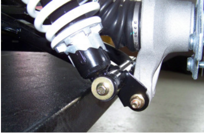
Fig. 9: Shock absorber mounting
