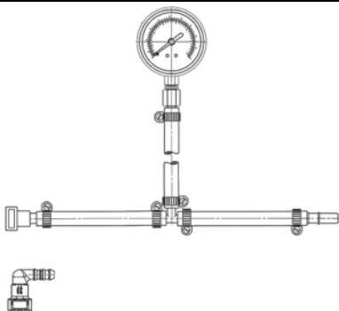
■ **NOTE:** When testing fuel pressure on the Sno Pro 500 models, remove the straight fuel pump connector and install 90° Fuel Pump Connector.
