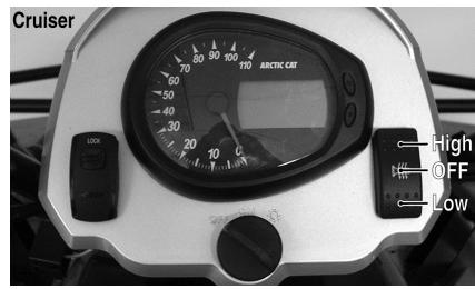
The passenger's handwarmers are controlled by a rocker-type switch located beneath the right-side handgrip. There are three positions on the switch (Low/Off/High).
