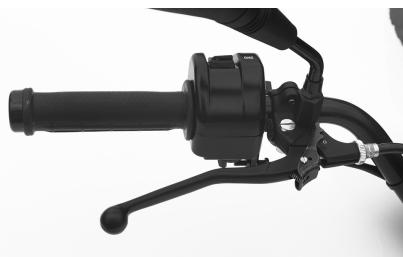
To engage and release the emergency/parking brake, use the following procedure.
