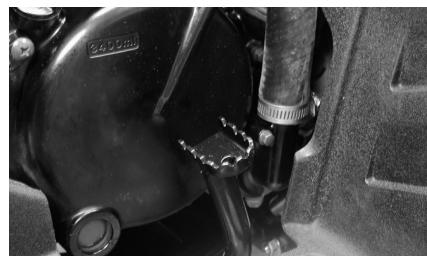
Pressing the foot brake pedal downward will apply brakes to all wheels.
