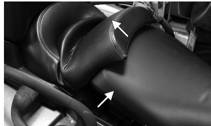
1. To remove the front seat, pull the seat lock lever up (located at the rear of the seat). Raise the rear end of the seat and slide it rearward.
