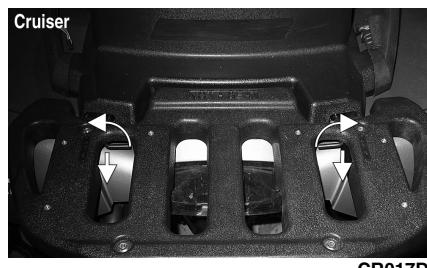
2. Lift the rear of the seat up; then pull slightly to the rear and lift the seat off the mountings.
