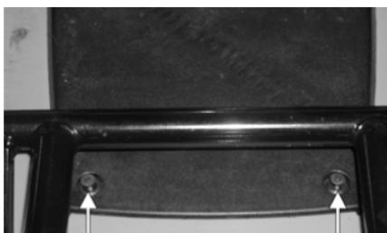
2. Lift the front of the access panel; then slide the panel forward to disengage the two rear tabs.
