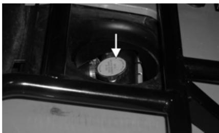
5. Add coolant as necessary; then install the radiator cap and access panel.
