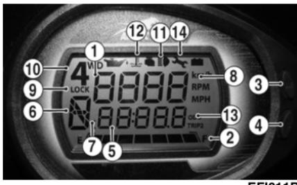
1. Speedometer/Tachometer/Condition Warning Display - Indicates the approximate vehicle speed (MPH or km/h) or RPM. Warns of a system error condition requiring attention.
