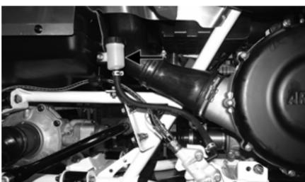
■ **NOTE:** The brake fluid reservoir is located in the right rear fender well.
