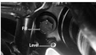
1. With the ATV on level ground, remove each oil filler plug.
