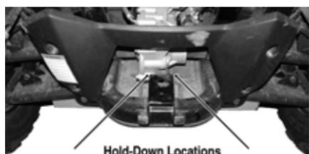
■ **NOTE:** Suitable hold-down straps are available from your Arctic Cat dealer. Ordinary rope is not recommended because it can stretch under load.
