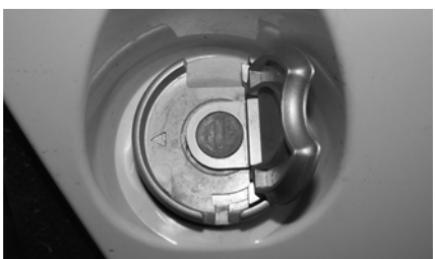
2. After filling the tank, position the lid towards the right side of the filler neck and rotate the lid  $\frac{1}{4}$  turn clockwise to secure. Flip the lid up.
