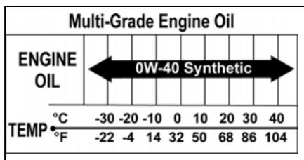
**■ NOTE:** If the vehicle will be operated under severe conditions (heavy pulling or loading, extremely high ambient air temperatures, or extended high-speed operation), Arctic Cat recommends installing an engine oil cooler kit if not so equipped. For additional information, see your local authorized Arctic Cat dealer.
