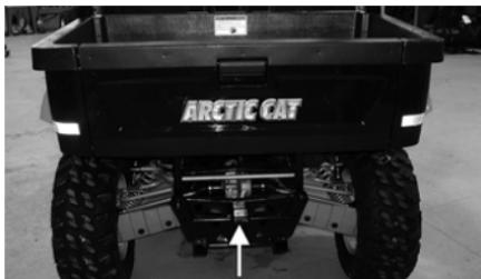
This vehicle is equipped with a rear frame-mounted receiver for a standard 5.1 cm (2 in.) receiver hitch. The standard receiver hitch must be purchased separately.
