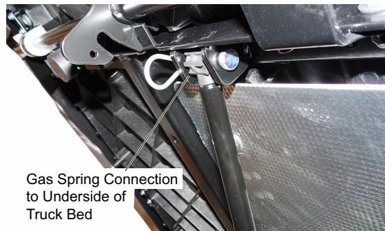
Gas Spring Connection to Underside of Truck Bed
