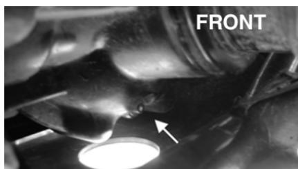
3. After the oil has been drained, install the drain plugs and tighten to 45 in.-lb (front) and 16 ft-lb (rear).
