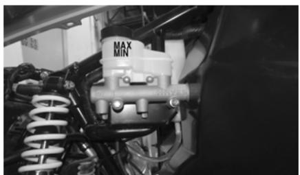
**■ NOTE: The brake fluid reservoir is located on top of the master cylinder above and to the rear of the front left wheel.**
