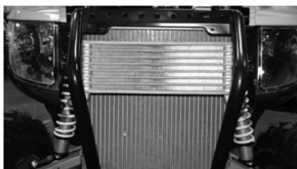
■ NOTE: Dirt and debris must be cleaned from the cooling fins regularly to ensure proper engine oil cooling.
