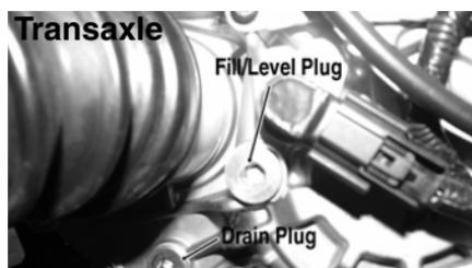
2. Drain the oil into a drain pan by removing the drain plugs.
