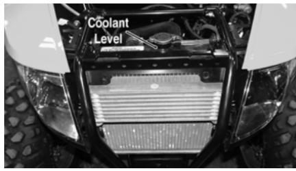
■ NOTE: Ensure coolant level is between the MAX and MIN marks of the overflow bottle.
