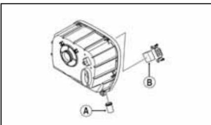
13. Install the air filter, cover, drain, and crankcase breather filter.
