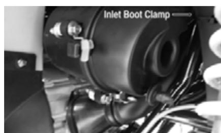
2. Remove the filter housing cover and air filter element.
