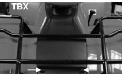
2. On the TBX, lift the front of the access panel; then slide the panel forward to disengage the two rear tabs; then move the panel rearward until free of the rack.
