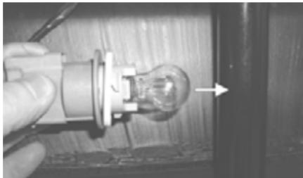
4. Insert the socket into the housing and rotate it clockwise.
