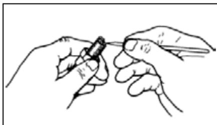
A light brown insulator indicates that the plug is correct. A white or dark-colored insulator indicates that the engine may need to be serviced. Consult an authorized dealer if the plug insulator is not a light brown color. Adjust the gap to specified amount (see specifications chart) for proper ignition. Use a feeler gauge to check the gap.
