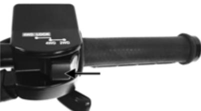
This switch allows the operator to operate the ATV in either two-wheel drive (rear wheels) or four-wheel drive (all wheels). For normal riding on flat, dry, hard surfaces, two-wheel drive should be sufficient. In situations of aggressive trail conditions, four-wheel drive would be the desired choice.
