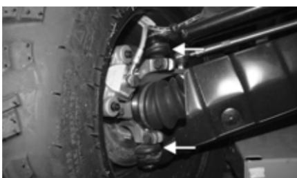
1. Secure the ATV on a support stand to elevate the front wheels.
