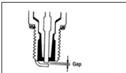
A new spark plug should be tightened 1/2 turn once the washer contacts the cylinder head. A used spark plug should be tightened 1/8 - 1/4 turn once the washer contacts the cylinder head.
