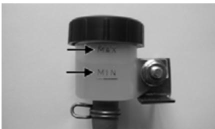
■ **NOTE: The brake fluid reservoir is located under the seat.**
