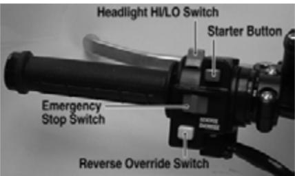
Use the headlight HI/LO switch to select the high or low headlight beam when the ignition switch is in the LIGHTS position. When the switch is in the HI position, the high beam will illuminate. When the switch is in the LO position, the low beam will illuminate.
