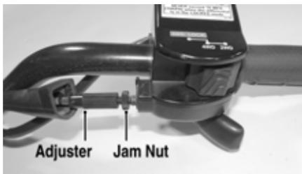
3. Tighten the jam nut against the throttle cable adjuster securely; then slide the rubber boot over the adjuster.
