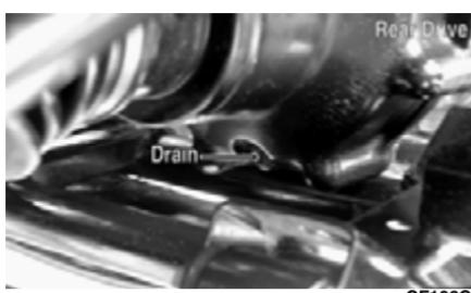
4. After all the oil has been drained, install the drain plugs and tighten to 45 in-lb.
