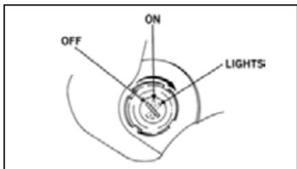
**OFF** position — All electrical circuits except the accessory plug are off. The engine will not start. The key can be removed in this position.
