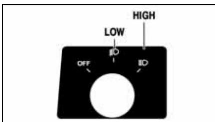
With the ignition switch in the RUN position, use the headlight switch to select low beam or high beam. The taillights work in all positions except OFF. The brake lights work in all light positions.
