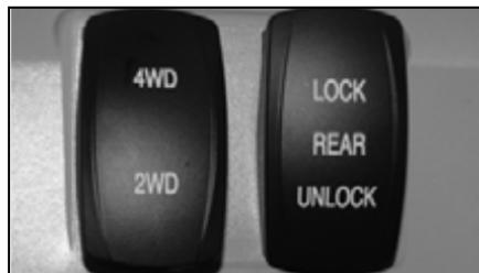
To select 2WD, depress the bottom of the 2WD/4WD switch. To select 4WD, move the switch to the opposite position. To engage the rear axle lock, push the top of the rear axle lock switch.
