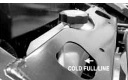
■ NOTE: If you cannot see any coolant in the reservoir, inspect the cooling system for leaks. If no leaks are present, add coolant using the bleed procedure below. If a coolant leak is suspected, schedule service with an Authorized Dealer.
