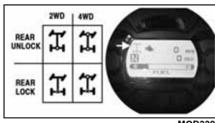
**■ NOTE:** Maneuverability and handling characteristics will differ with the rear axle lock engaged.
