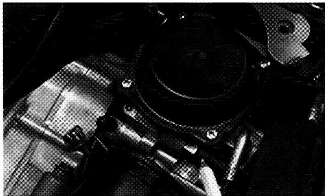
6. Connect the fuel supply hose to the carburetor; then turn the gas tank valve to ON. Check for leakage.
