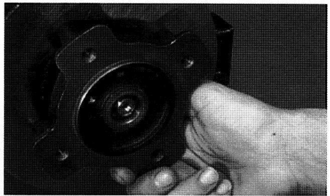
9. Insert the hub seal onto the shaft; then position it into the hub.
