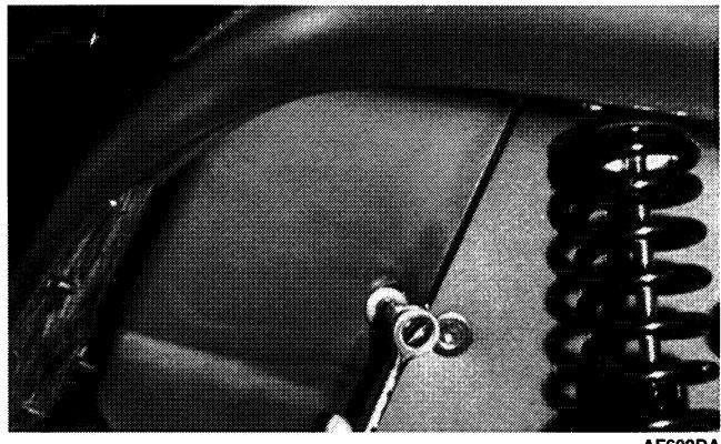
2. Tighten the machine screws securely.
