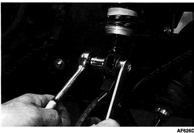
10. Remove the cap screws securing the A-arm to the frame.
