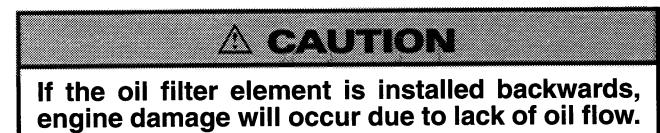
7. Place the filter cover in position and secure with the nut. Tighten securely.
