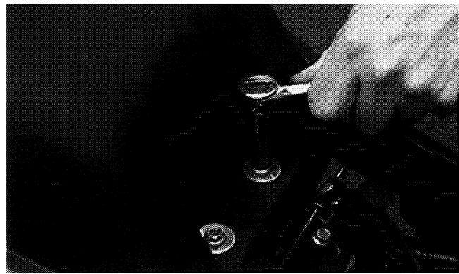
5. Remove the cotter pin and slotted nut securing each tie rod end to the steering post actuator arm. Remove the tie rod ends from the arm.
