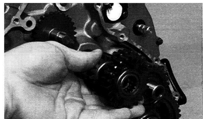
15. Remove the #2 gear and the select sliding dog gear from the driveshaft.
