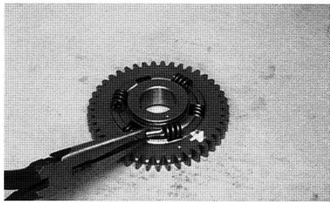
4. Install the thrust washer and spring washer (with its raised inner portion directed away from the gear); then install the circlip with the sharp edge facing away from the gear.
