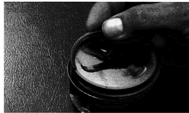
2. Remove each ring by working it toward the dome of the piston while rotating it out of the groove.
