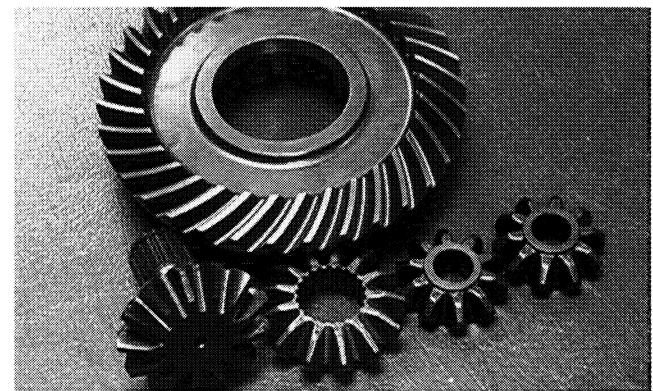
36. Remove the right-side gear from the differential case and account for washer(s).
