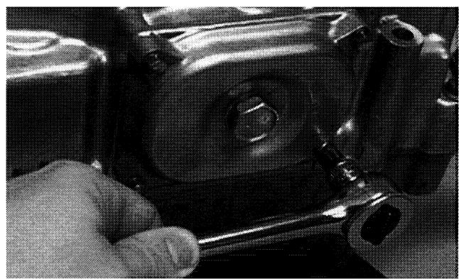
3. Place the oil pump into position in the crankcase and secure with the three Phillips-head screws coated with blue Loctite #242. Tighten to 1 kg-m (7 ft-lb).
