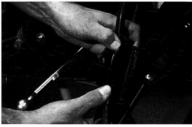
4. Secure the lower eyelet of the shock absorber to the upper A-arm. Tighten nut to 4.8 kg-m (35 ft-lb).
