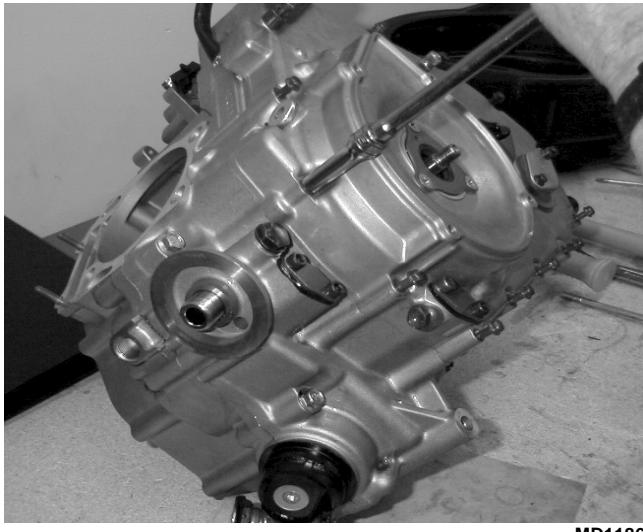
4. Using Side Case Puller (p/n 0644-262) and the 6 mm adapter, remove the left-side cover w/stator assembly. Note the condition of the gasket. Replace if necessary. Account for the two alignment pins and the position of the shifter bracket for installing purposes.
