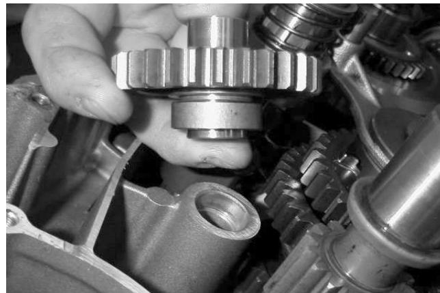
11. Install the secondary (4x4 models) and primary driveshaft assemblies. Account for the bearing alignment C-ring on the bearing boss next to the pinion gear.
