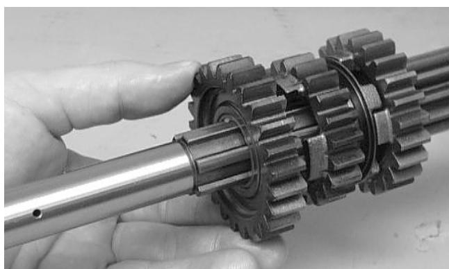
3. Remove the 5th drive washer and 5th drive circlip from the countershaft.
