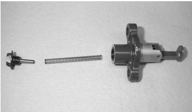
20. Depress the spring-loaded lock and push the plunger into the tensioner.
