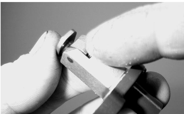
21. Place the chain tensioner adjuster assembly and gasket into position on the cylinder making sure the ratchet side is facing toward the top of the cylinder and secure with the two Allen-head screws.
