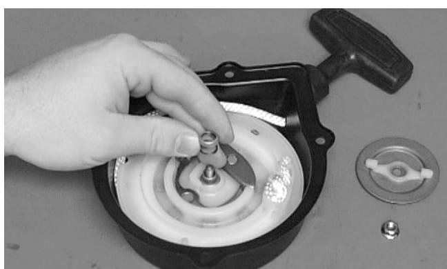
8. Install the friction plate with the ratchet guide fitting into the ratchet.
