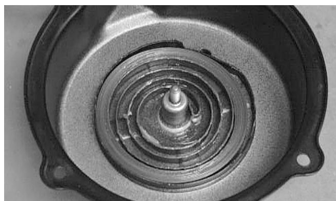
2. Insert the rope through the hole in the reel and tie a knot in the end; then wrap the rope counterclockwise around the reel leaving approximately 50 cm (20 in.) of rope free of the reel.
