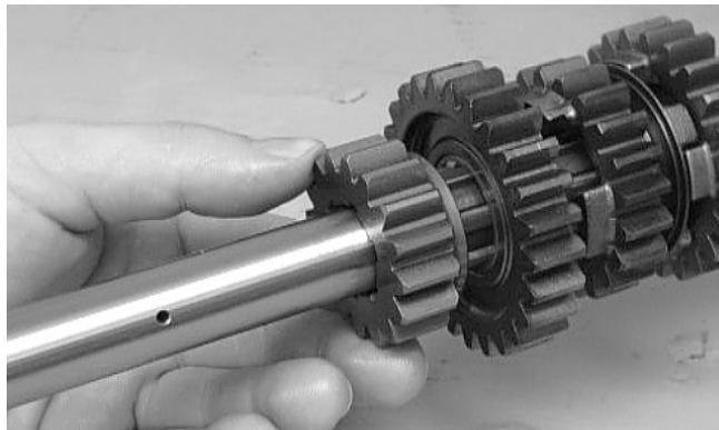
2. Remove the 5th drive gear from the countershaft.
