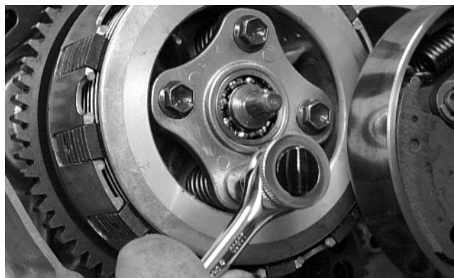
3. Remove the release roller assembly. Account for four springs.
