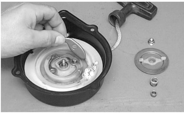
7. Carefully lift the reel free of the case making sure the spiral spring does not accidentally disengage from the case.
