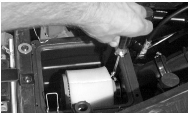
6. Place the air cleaner cover into position and secure with the retaining clips.
