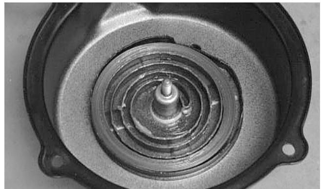
2. Insert the rope through the hole in the reel and tie a knot in the end; then wrap the rope counterclockwise around the reel leaving approximately 50 cm (20 in.) of rope free of the reel.
