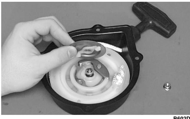
9. While pushing down on the reel, install the nut. Tighten securely.
