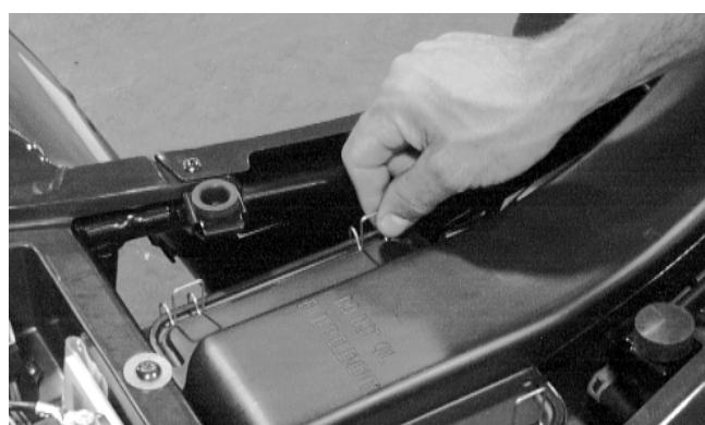
3. Loosen the clamp and remove the filter.
