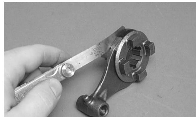
3. Shift fork to groove side clearance must be within specifications.
