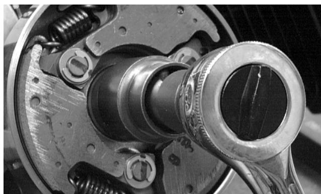
■ NOTE: It will be necessary to remove the lower rear oil filter cover stud and the upper arm cap screws to provide clearance for removing the cover.
