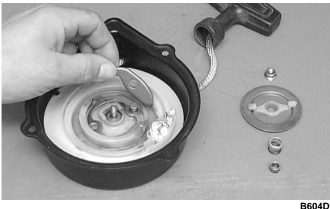
7. Carefully lift the reel from the case making sure the spiral spring does not accidentally disengage from the case.
