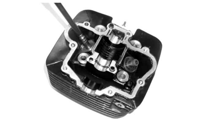
4. After installing the guide, use the standard valve guide reamer to remove all burrs and tight areas that may remain in each valve guide.
