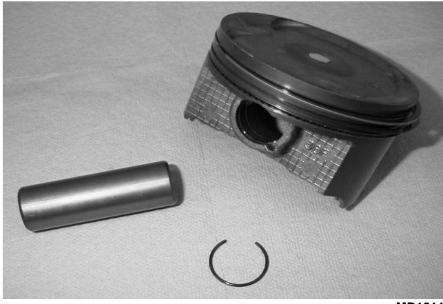
A. Starting with the top ring, slide one end of the ring out of the ring-groove.
