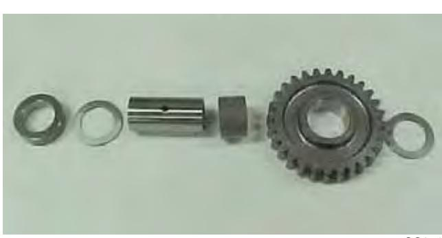
10. Install the washer, spacer, sleeve, reverse idler gear, and washer.
