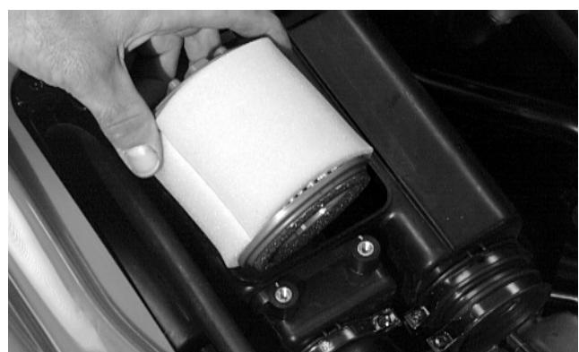
4. Fill a wash pan larger than the filter with a non-flammable cleaning solvent; then dip the filter in the solvent and wash it.
