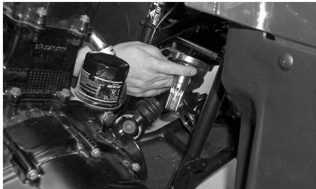
3. Position the two upper rear engine mounts in place on the frame and loosely secure with existing hardware; then install the three engine mounting through-bolts making sure to account for a washer on the upper bolt and a spacer on the lower front bolt. Tighten only until snug.
