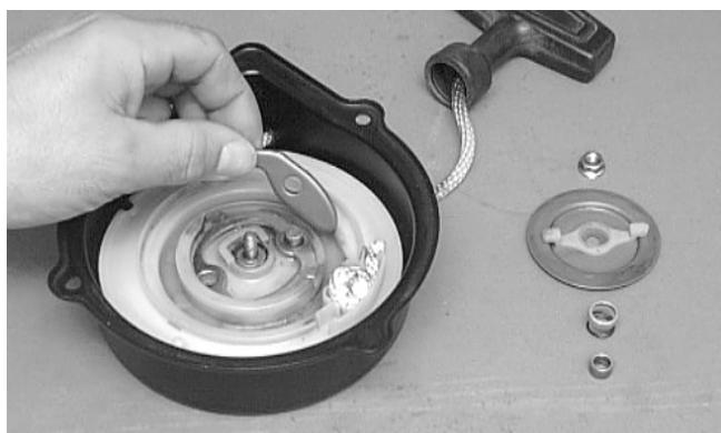
7. Install the shaft, spring, and the spring cover.
