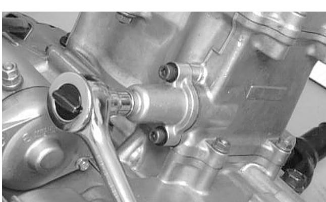
23. Rotate the crankshaft until the first cap screw securing the sprocket to the camshaft can be installed; then install the cap screw. Do not tighten at this time.
