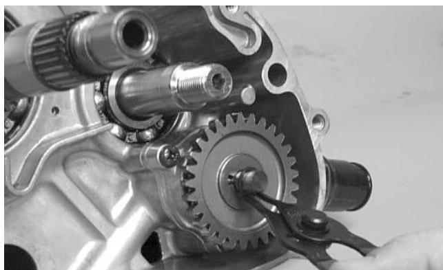
5. Place the gear shift cam plate and guide onto the gear shift cam making sure the alignment pin was installed. Secure assembly with the cap screw coated with blue Loctite #243. Tighten securely.
