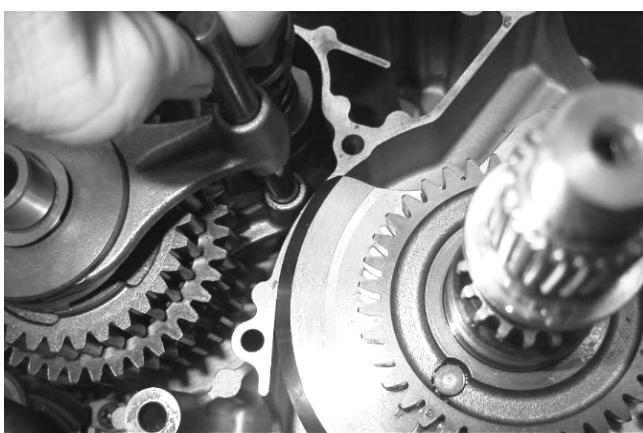
9. Install the input driveshaft.
