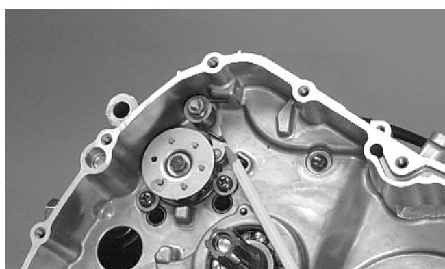
7. Install the gear shift shaft.
