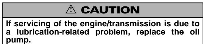
■ NOTE: For general servicing, it is advisable to disassemble, clean, and inspect the oil pump. If any wear or damage is suspected, replace the oil pump.
