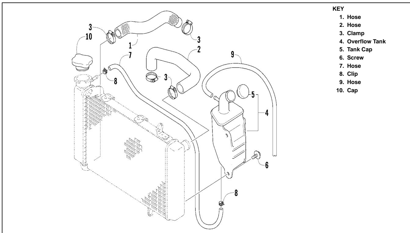
The cooling system capacity is approximately 1.2 L (1.3 U.S. qt). The cooling system should be inspected daily for leakage and damage. Also, the coolant level should be checked periodically.
