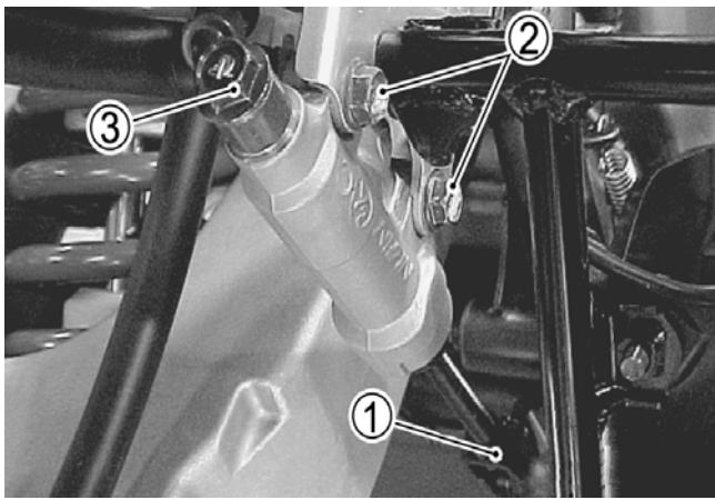
5. Install the reservoir tank hose; then fill the master cylinder reservoir with DOT 4 brake fluid and bleed the system. See Section 2.
