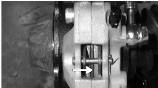
3. If thickness of any brake pad is less than 2.0 mm (0.078 in.), all brake pads must be replaced.
