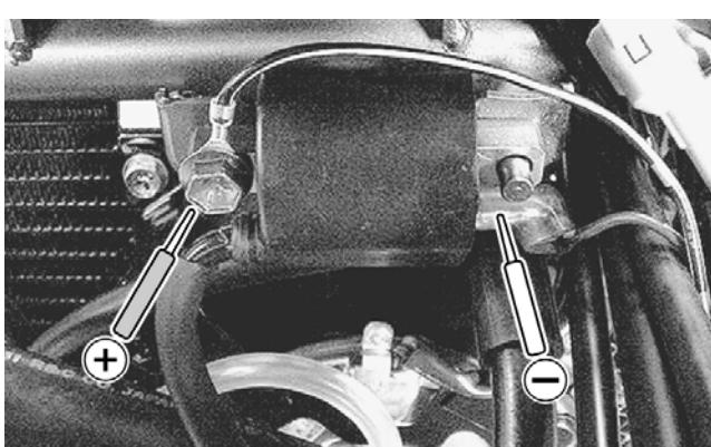
3. Set the meter selector to the D.C. Voltage position.
