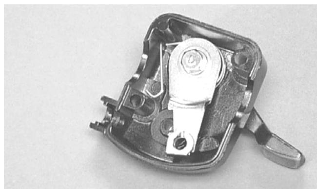
2. Using a pair of needle-nose pliers, place the spring into position on the actuator arm.
