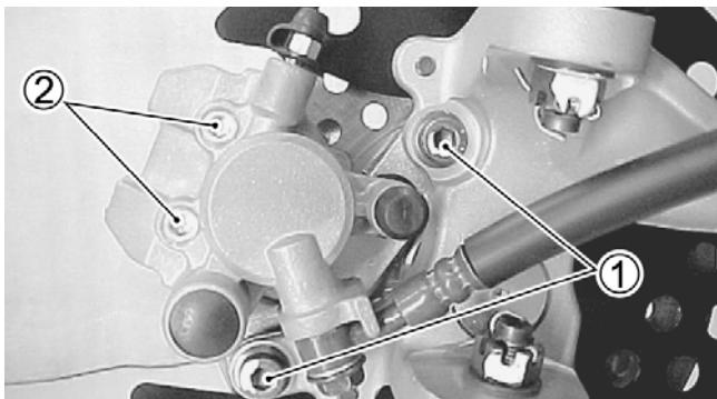
**■NOTE: Do not compress the brake lever after the brake pads are removed.**
