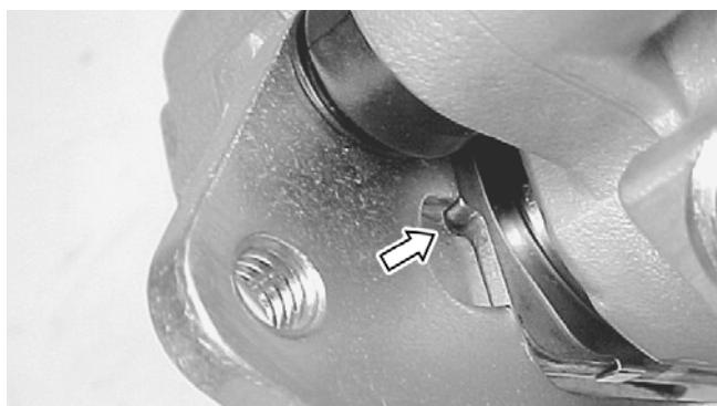
5. Install the new brake pads; then tighten the brake pad mounting pins and the brake caliper mounting cap screws to specifications.
