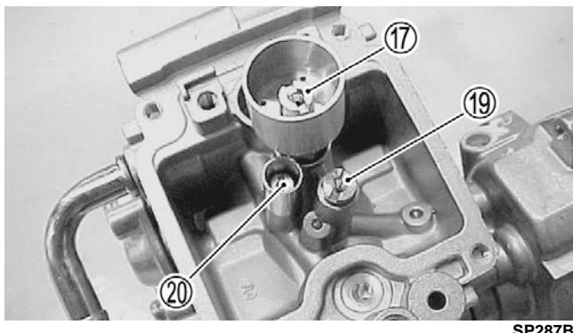
4. Place the float assembly (with needle valve) into position and secure to the carburetor with the float pin.
