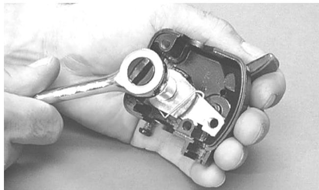
4. Remove the actuator arm and account for a bushing. Note the position of the return spring for installing purposes.
