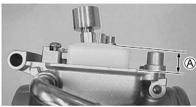
5. Place the float chamber into position making sure the O-ring is properly positioned; then secure with the Phillips-head screws.
