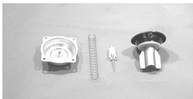
8. Place the diaphragm cover into position; then secure with the Phillips-head screws. Tighten securely.
