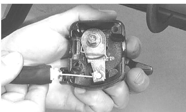
3. Remove the cap screw, lock washer, and washer securing the actuator arm to the throttle control lever.
