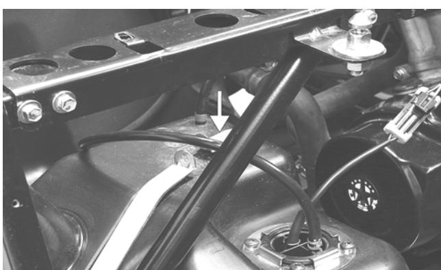
2. Swing the front hold-down to the right into position and install the cap screw and nut. Do not tighten at this time.
