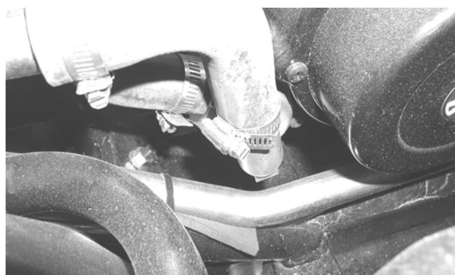
5. Remove the two cap screws securing the water pump to the engine; then remove the water pump.
