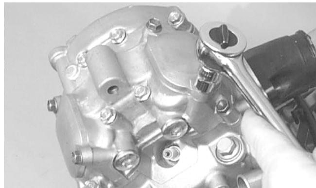
■NOTE: Keep the mounting hardware with the covers for assembly purposes or thread them back into the head to keep them separated.
