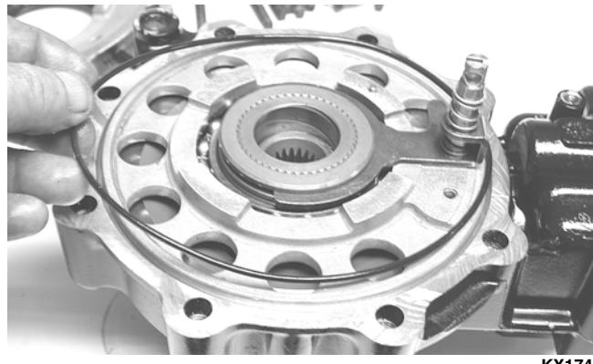
■**NOTE:** If the cover is difficult to remove, pry on the cover in more than one recessed location.
