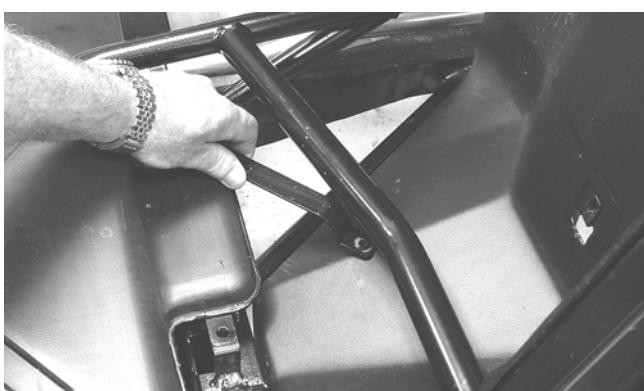
3. Install the rear hold-down strap joining cap screw and nut. Do not tighten at this time.
