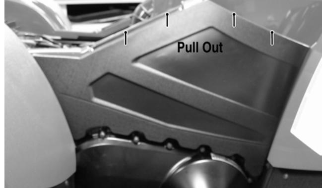
5. Remove the instrument pod; then remove the front rack and front body panel (see Steering/Frame/Controls).
