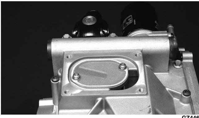
2. Remove the cap screws securing the lower crankcase to the upper crankcase halves; then using a rubber hammer, free the lower crankcase and remove. Account for two alignment pins.
