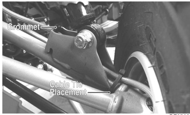
4. Secure the lower eyelet of the shock absorber to the upper A-arm. Tighten nut to 50 ft-lb.
