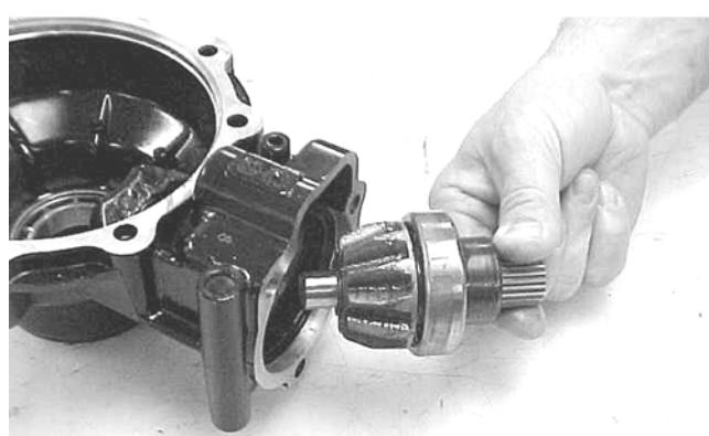
3. Secure the pinion gear in a bearing puller; then remove the pinion bearing using a press. Account for a collar and a bearing.
