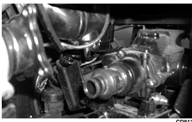
28. Remove the block from under the engine and lower the engine; then remove the boot clamp from the front output drive yoke.
