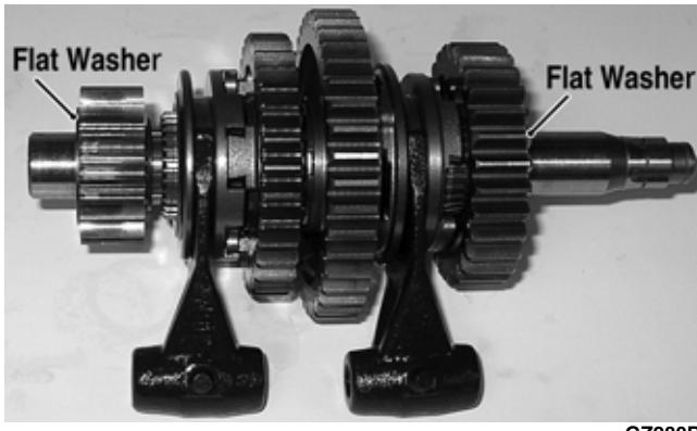
8. Remove the reverse idler gear (I), shaft bushing, and two washers.
