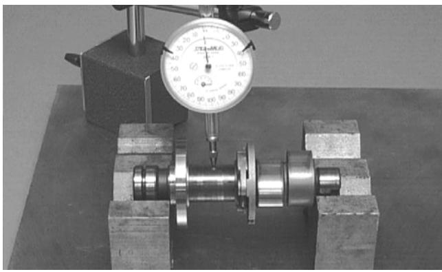
2. Rotate the camshaft and note runout; maximum tolerance must not exceed specifications.
