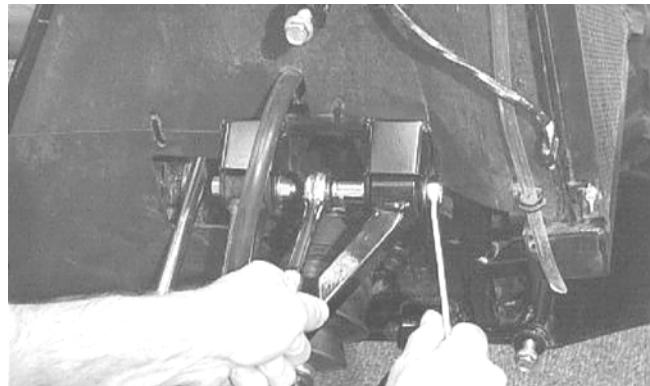
3. Route the brake hose through the upper A-arm shock absorber mount; then secure the hose to the A-arm with a cable tie and grommet.
