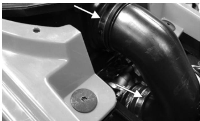
6. Remove the air inlet and outlet ducts from the CVT housing.
