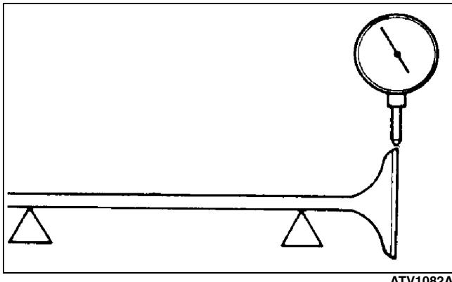
3. Rotate the valve in the V blocks.
