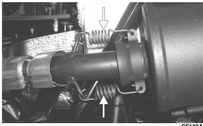
2. Slide the muffler rearward to clear the mounting lugs and remove the muffler.
