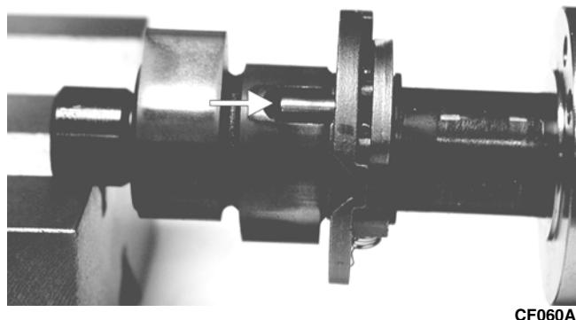
2. If damaged, the camshaft must be replaced.
