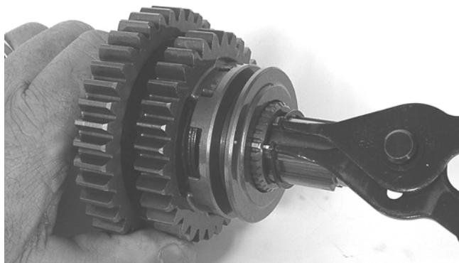
3. Remove the reverse driven gear dog.
