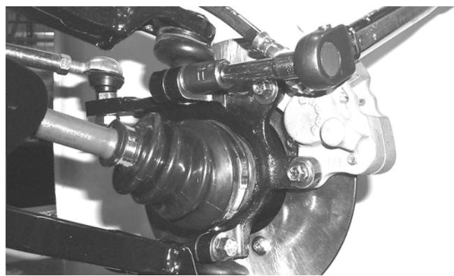
7. Install the tie rod end and secure with the nut. Tighten to 30 ft-lb; then install a new cotter pin and spread the pin to secure the nut.
