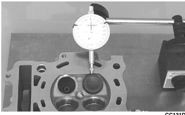
3. Push the valve from side to side; then from top to bottom.
