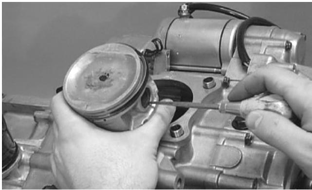
17. Using the Piston Pin Puller, remove the piston pin. Account for the opposite-side circlip. Remove the piston.
