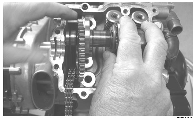
**■NOTE: At this point, oil the camshaft bearings, cam lobes, and the three seating journals on the cylinder.**
