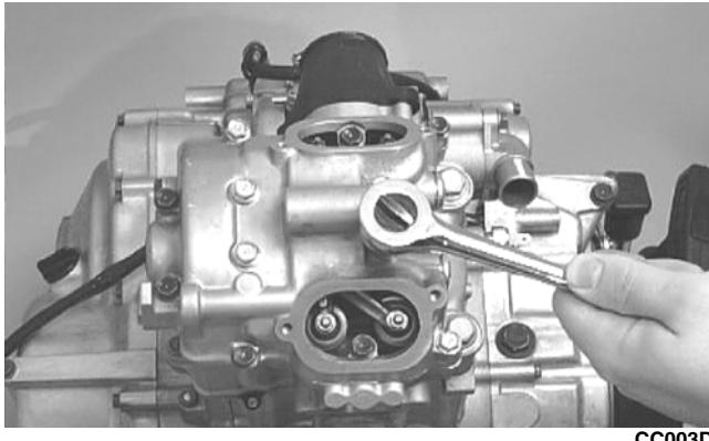
30. In a crisscross pattern starting from the center and working outward, tighten the cap screws (from step 29) to 8.5 ft-lb.
