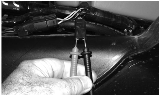
3. The meter must show battery voltage.
