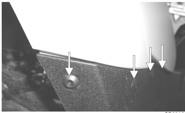
2. Remove the screws securing the foot pegs to the footrests; then remove the foot pegs and footwells.
