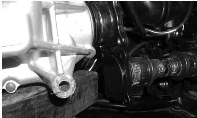
27. Remove the first small boot clamp; then remove the output flange and driveshaft from the rear drive coupler.
