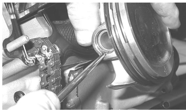
2. Place the two alignment pins into position. Place the cylinder gasket into position with a drop of silicone sealant at the front and rear crankcase junction; then place a piston holder (or suitable substitute) beneath the piston skirt and square the piston in respect to the crankcase.
