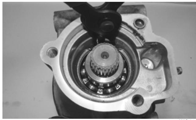
2. Using the Pinion Gear/Shaft Removal Tool and a hammer, remove the pinion gear from the gear case housing.
