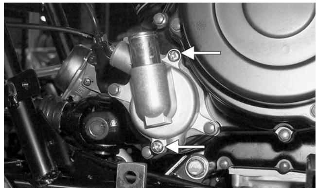
6. Remove the two cap screws securing the water pump to the engine; then remove the water pump.
