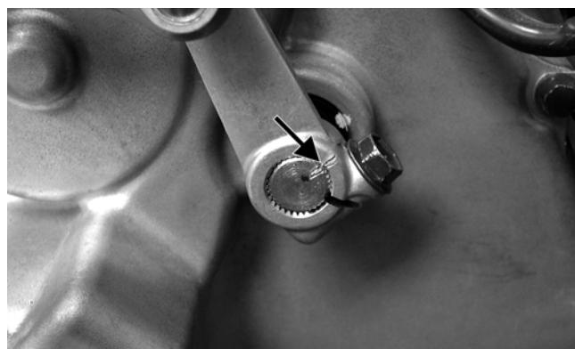
4. Remove the cap screws securing the speed sensor housing to the crankcase and remove the housing assembly; then remove the snap ring securing the speed sensor trigger to the shaft and remove the trigger. Account for the gasket.
