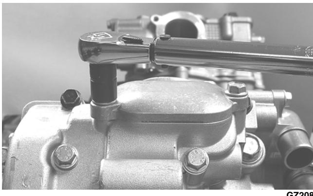
39. If removed, install the spark plugs. Tighten securely.
