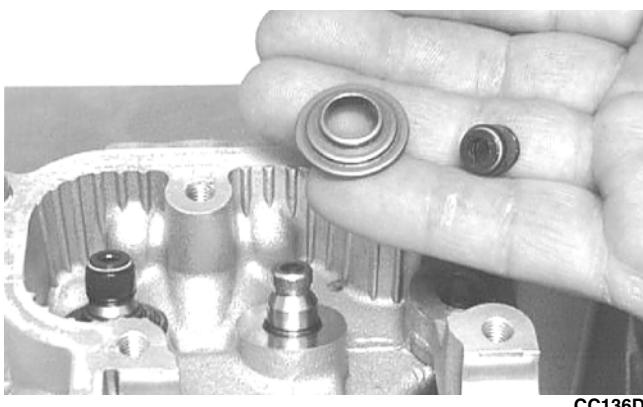
**■NOTE:** The valve seals must be replaced.
