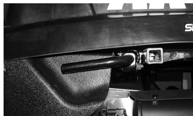
2. Remove the nut from the lower end of the box lift support.
