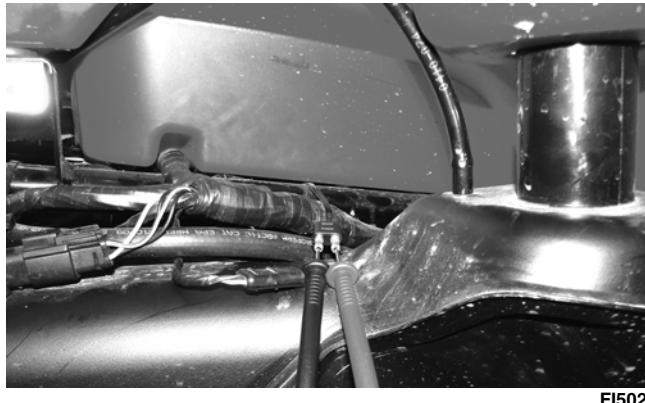
3. When the brake pedal is depressed, the meter must show less than 1 ohm.
