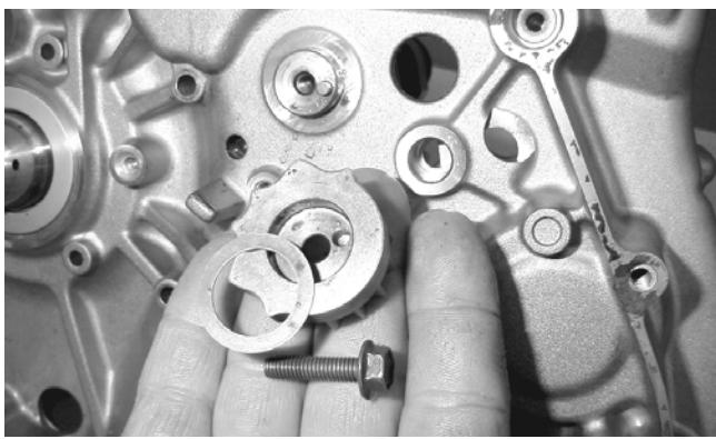
4. Install the shift detent cam arm and spring.
