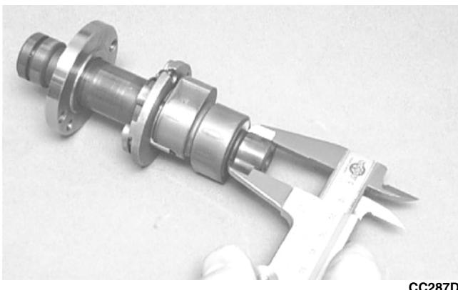
**■NOTE:** If the journals are worn, replace the camshaft; then measure the clearance again. If it is still out of tolerance, replace the cylinder head.
