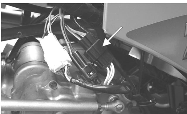
■NOTE: Test the connector that comes from the engine.
