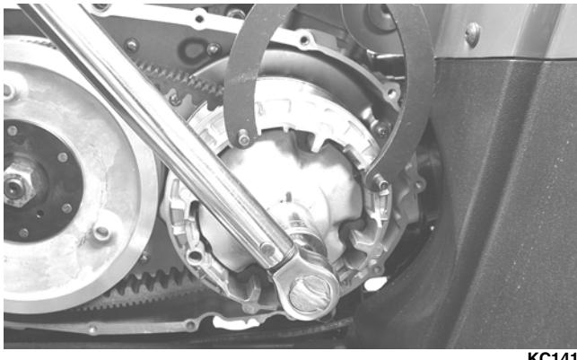
■**NOTE:** At this point, the cap screw can be removed from the driven pulley face.
