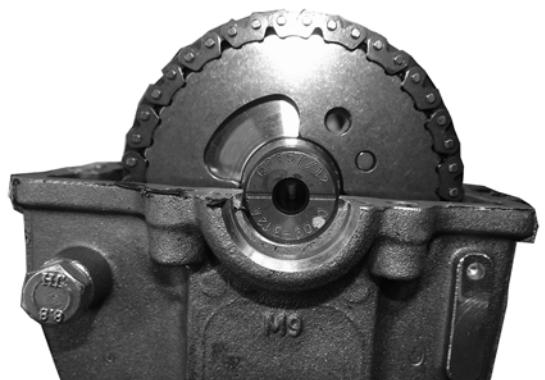
14. Seat the cam sprocket onto the camshaft making sure the alignment pin in the camshaft aligns with the smallest hole in the sprocket; then place the cam-shaft/sprocket assembly onto the cylinder ensuring the following.
