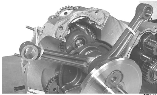
2. Coat both sides with engine oil; then install the spacer washer on the crankshaft with the radius directed toward the crankshaft.
