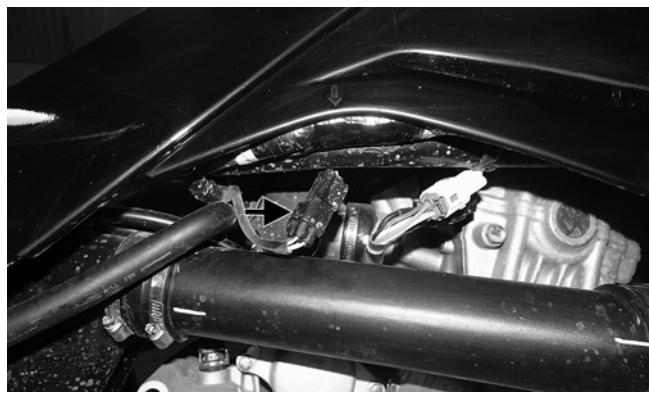
2. On the sensor side of connector, connect the black (negative) test lead to one white wire pin; then connect the red (positive) test lead to the other white wire pin.
