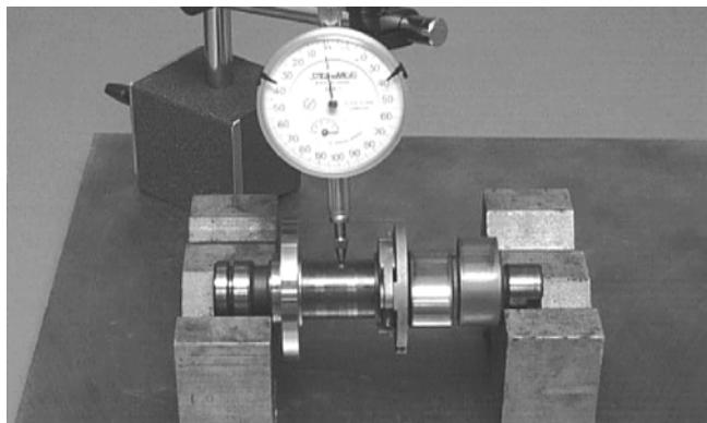
2. Rotate the camshaft and note runout; maximum runout must not exceed specifications.
