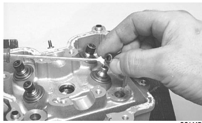
2. Insert each valve into its original location.
