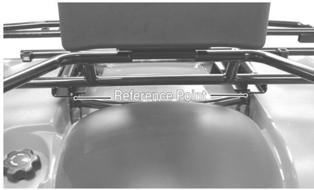
5. Adjust the handlebar direction until the two measurements are equal; then secure the handlebar to the rear rack using tie-down straps.
