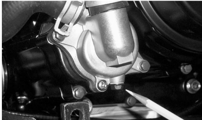
2. Drain the oil from the engine/transmission.
