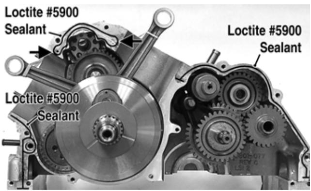
4. Carefully join the crankcase halves by placing the left-side crankcase onto the assembled right side. Secure with the cap screws (eight left side and one right side).
