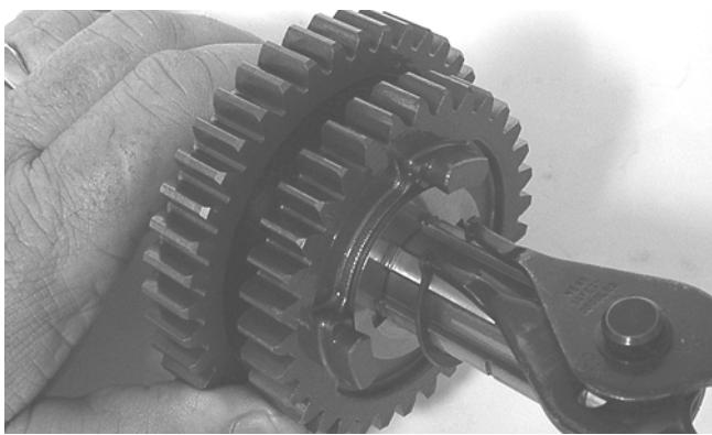
5. Remove the reverse driven washer; then remove the low driven gear locking washer.
