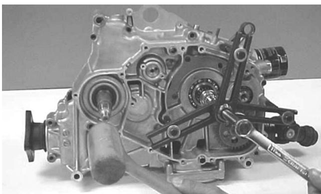
■**NOTE:** To keep the shaft/gear assemblies intact for identification, tap the shafts toward the left-side crankcase half when separating the halves.
