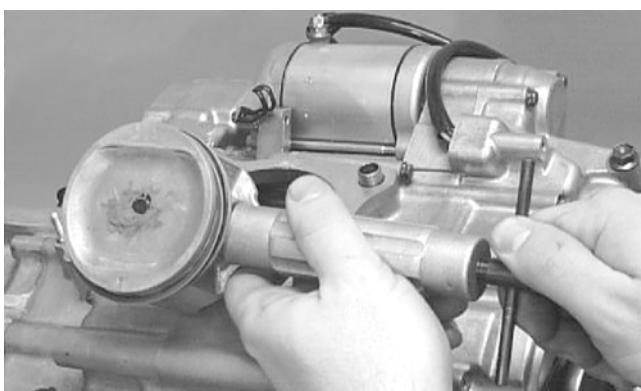
■**NOTE:** Support the connecting rod with rubber bands to avoid damaging the rod or install the Connecting Rod Holder.
