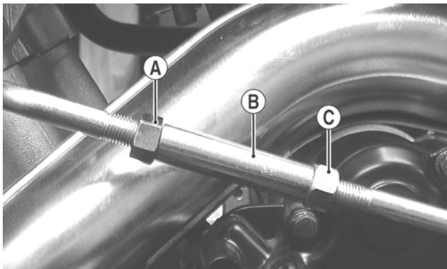
3. Tighten the jam nuts securely; then shift the transmission to each position and verify correct adjustment.
