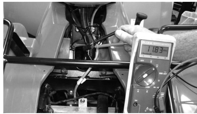
3. The meter must show battery voltage.
