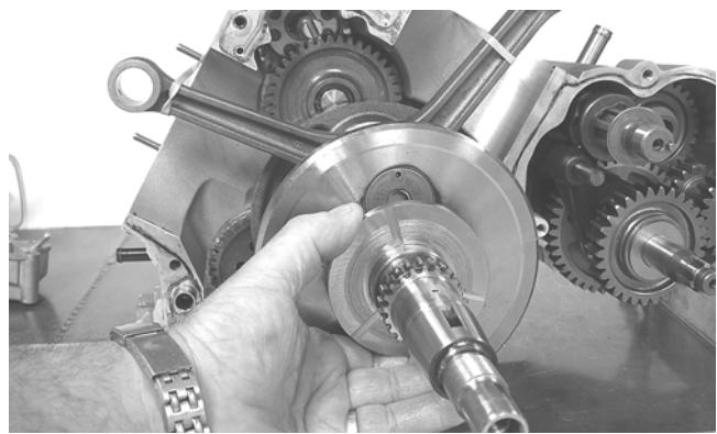
3. Install the two alignment pins; then apply a thin bead of Loctite #5900 or suitable substitute sealant to the crankcase mating surface.
