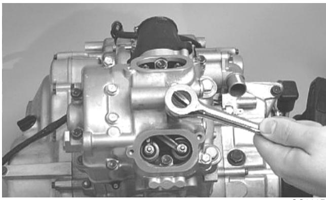
36. In a crisscross pattern starting from the center and working outward, tighten the cap screws on both valve covers to 8.5 ft-lb.
