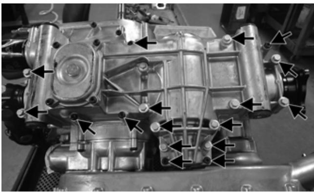
3. Remove the secondary drive assembly; then remove the secondary driven shaft assembly and set aside. Account for one locating ring.
