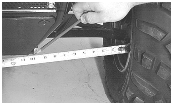
**■NOTE: The distances from the inside rims to the frame tubes should be equal. If the measurements are equal, proceed to step 8; if the measurements are not equal, proceed to step 7.**
