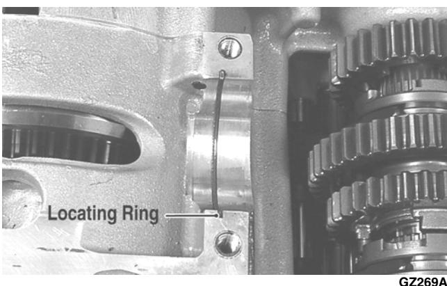
■NOTE: Do not disassemble these assemblies unless service is required. If disassembled, secondary gear sets will have to be reset for backlash and gear contact (see Servicing Center Crankcase Components sub-section).
