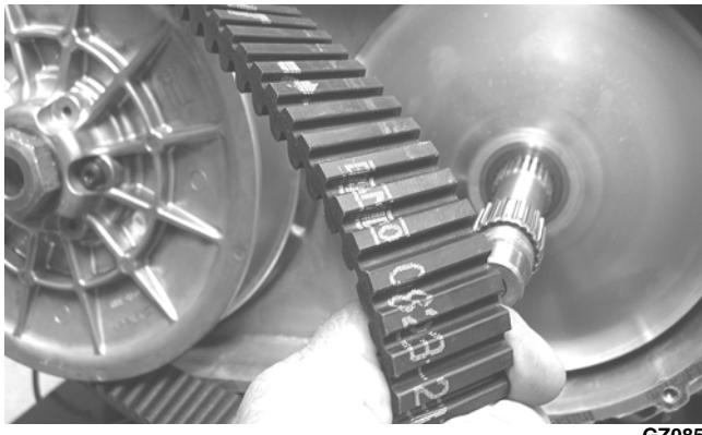
■**NOTE: The arrows on the V-belt should point forward.**
