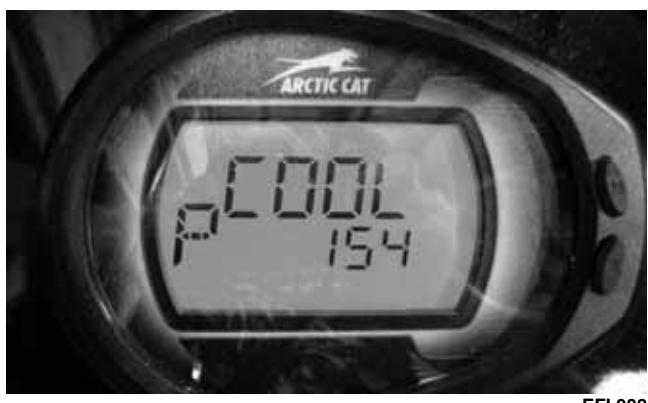
Display: Engine coolant temperature as measured by the ECT sensor.
