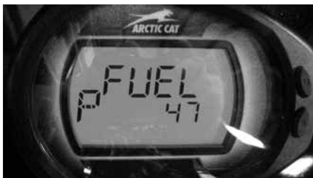
Display: Fuel level signal from the fuel level sensor (measured in ohms).
