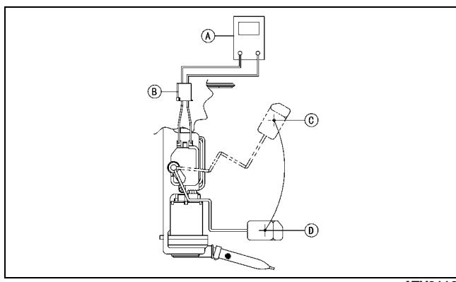
■**NOTE:** If readings are erratic, clean the resistor wiper and resistor with clean alcohol and retest. If still not correct, replace the fuel level sensor.
