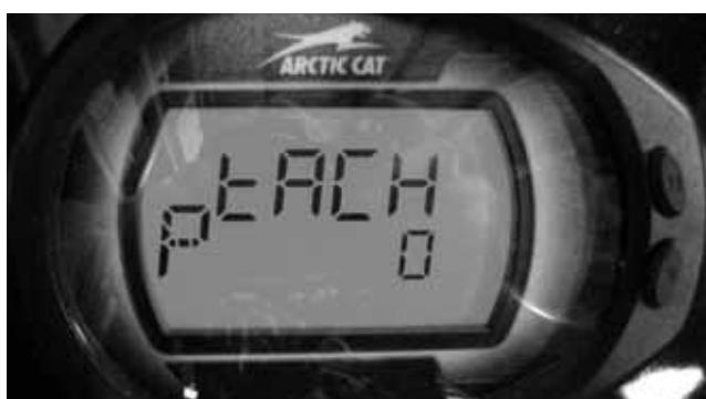
Display: Engine RPM
