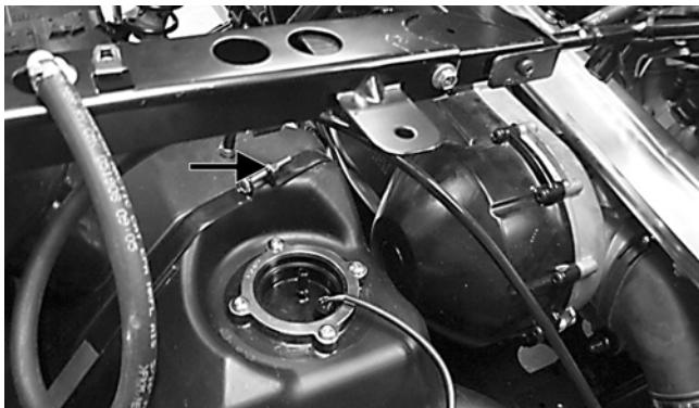
6. Lift and slide the tank forward raising the front of the tank first; then turn the tank and lift out the right side.
