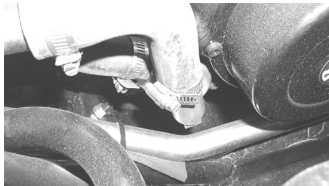
5. Remove the two cap screws securing the water pump to the engine; then remove the water pump.
