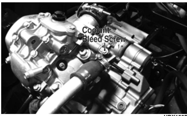
**■NOTE:** While the cooling system is being filled, air pockets may develop; therefore, run the engine for five minutes after the initial fill, shut the engine off, and then fill the cooling system.
