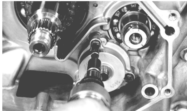
3. Install the oil pump drive gear spacer onto the crank balancer shaft. Grease the pin and insert it into the shaft; then install the drive gear making sure the raised side of the gear is facing toward the inside. Secure the gear with the cap screw (threads coated with red Loctite #271) and the washer. Tighten the cap screw to 63 ft-lb.
