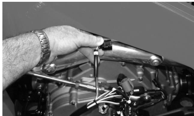
3. On the 500 using a multimeter, connect the black tester lead to the black socket (GND) on the analyzer and the red tester lead to the white socket (VAR); then select the DC Voltage position. With the vehicle off, the gauge should read 0.66-0.70 and at Wide-Open Throttle it should read up to approximately 3.88.
