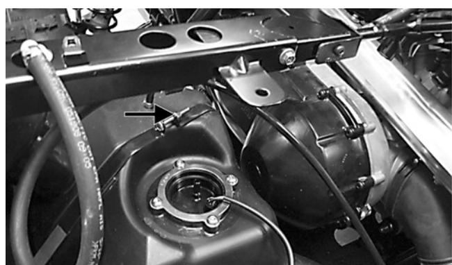
4. Place the gas cap filler panel into position; then if necessary, position the gas tank so the filler panel and filler neck are not binding or rubbing.
