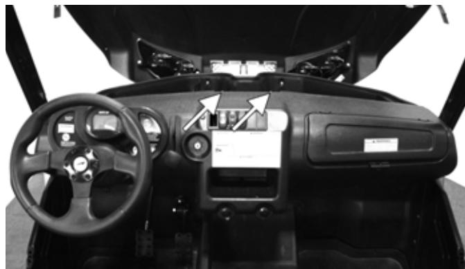
3. Remove the six sheet metal and three machine screws securing the dash assembly to the frame; then remove the shift lever grip and locking nut.
