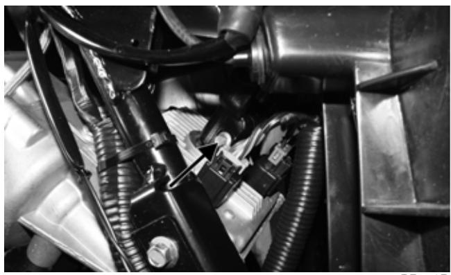
2. Install the steering shaft housing with steering shaft connecting the steering shaft and intermediate shaft first; then slide the housing into place on the steering support.
