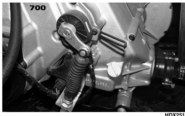
■NOTE: On the 500, shifting the transmission into park will aid in accessing the shift arm cap screw.
