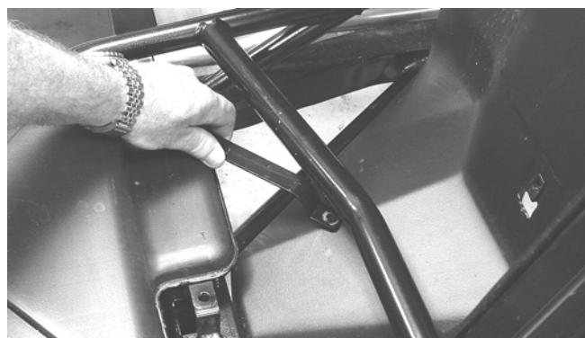
3. Install the rear hold-down strap joining cap screw and nut. Do not tighten at this time.
