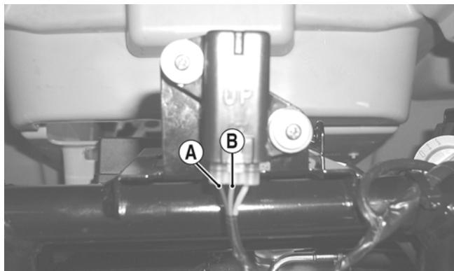
4. Tilt the sensor 60° or more to the left and right observing the meter. The meter should read 4.0-8.0 DC volts (700) or 3.0-7.0 DC volts (500) after approximately one second in the tilted position. If the meter readings are not as specified, the tilt sensor is defective.
