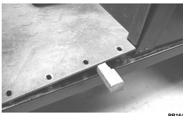
5. From the opposite side of the vehicle, repeat step 3; then lift the rear of the floor up and lift the floor out of the vehicle.
