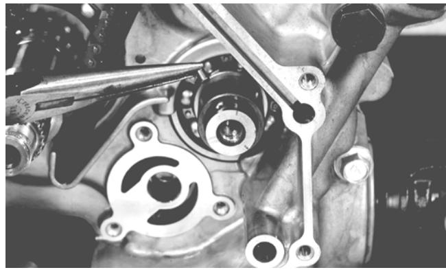
2. Install the oil pump onto the engine; then tighten the screws (coated with red Loctite #271) to 8 ft-lb.
