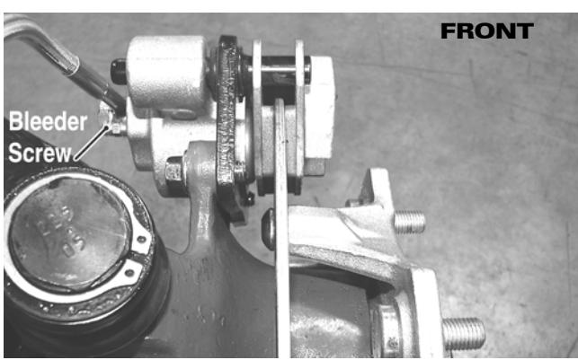
**■NOTE: During the bleeding procedure, watch the reservoir very closely to make sure there is always a sufficient amount of brake fluid. When the level falls below MIN, refill the reservoir before the bleeding procedure is continued. Failure to maintain a sufficient amount of fluid in the reservoir will result in air in the system.**
