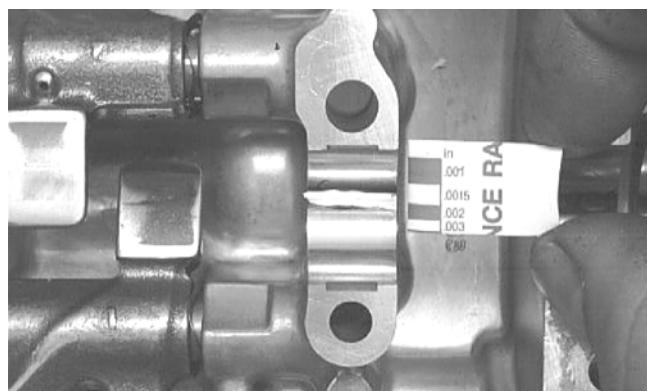
6. If clearance is excessive, measure the journals of the camshaft.
