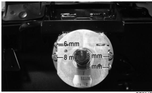
3. Install the cap screw in the intermediate shaft coupler and tighten to 31 ft-lb.
