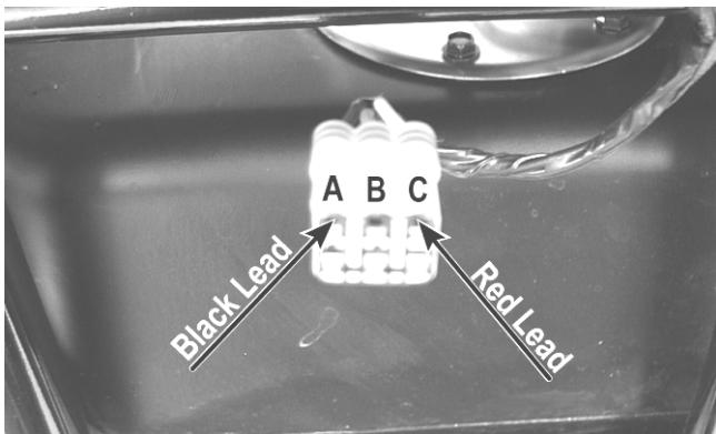
2. Turn the ignition switch to the ON position. The multimeter should read battery voltage. If battery voltage is not indicated, check the 30-amp fuse in the PDM or the 10-amp ignition fuse, wiring harness, or the ignition switch.
