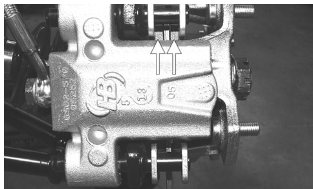
3. If thickness of either brake pad is less than 1.0 mm (0.039 in.), the brake pads must be replaced.
