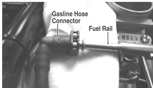
3. Turn the ignition switch to the ON position. The fuel pressure should build until the pump shuts off. Pressure should read 3.0 kg/cm<sup>2</sup> (43 psi).
