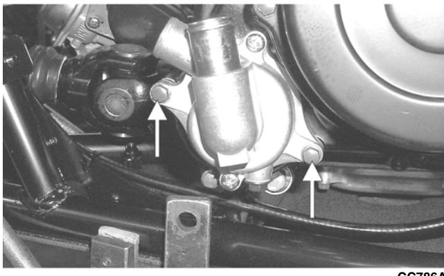
2. Connect the two coolant hoses to the water pump and secure with the clamps; then install the water pump coolant drain plug.
