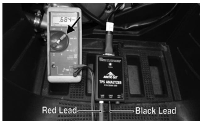
4. On the 700 using a multimeter, connect the black tester lead to the black socket (VAR) on the analyzer and the red tester lead to the white socket (+5V); then select the DC Voltage position. With the vehicle off, the gauge should read 0.58-0.62 and at Wide-Open Throttle it should read up to approximately 3.7.
