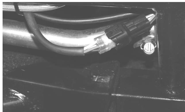
2. Connect the black lead to the black wire using a Maxi-Clip; then select 2WD on the drive select switch.
