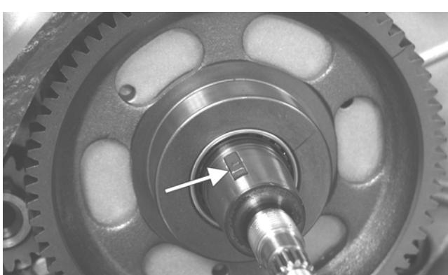
10. Remove the two starter gears from the crankcase noting the direction of the beveled side of the gears for installing purposes; then remove the two starter gear shafts.
