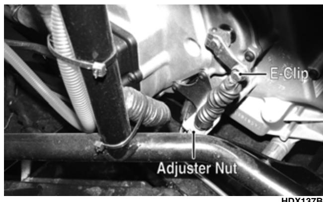
4. Remove the center floorboard and remove all nylon ties securing the cable housing to the frame; then remove the shift cable.
