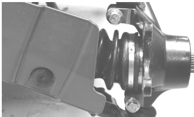
8. Tap the ball joint end out of the knuckle; then remove the knuckle.
