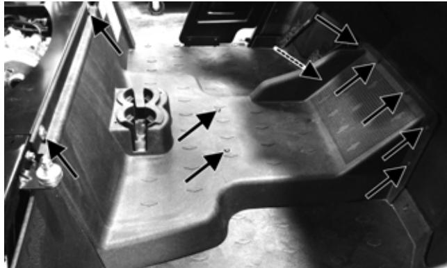
4. While pulling forward on the upper-rear of the floor, lift the rear part of the floor above the seat locating stud.
