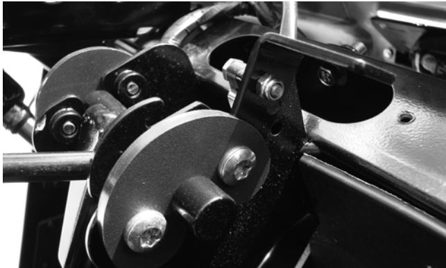
2. Secure the shift cable end to the shift arm stud with the cap screw and nut. Tighten to 8 ft-lb.
