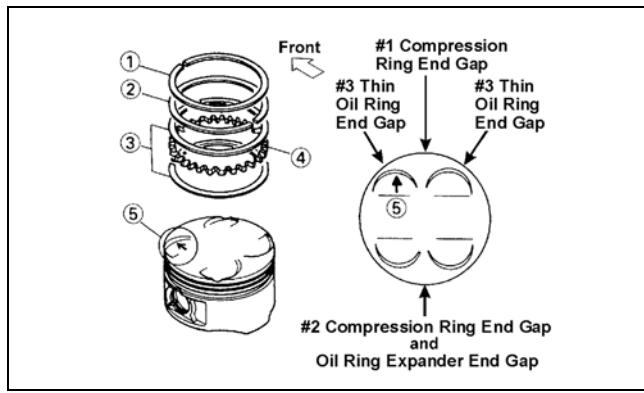
■NOTE: Note the direction of the exhaust side of the piston (5) for correct ring end gap orientation.
