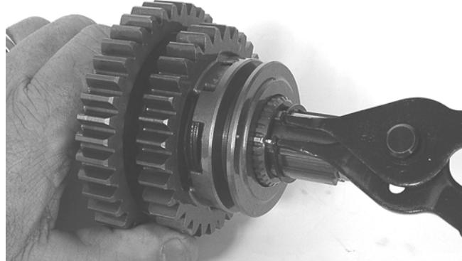
3. Remove the reverse driven gear dog.
