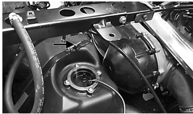
2. Swing the front hold-down to the right into position and install the cap screw and nut. Do not tighten at this time.
