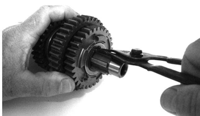
2. Remove the splined washer; then remove the reverse driven gear along with the bearing and bushing.
