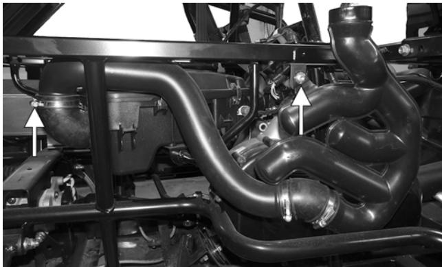
4. Remove the cap screws securing the support tube to the frame.
