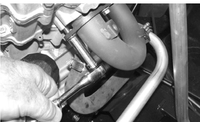
7. Install the O2 sensor and tighten the sensor to 19 ft-lb. Connect the harness to the sensor.
