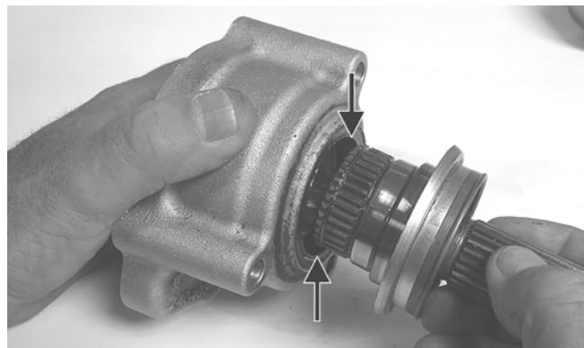
4. Using a new gasket, install the assembled rear drive input shaft/housing onto the rear drive gear case and secure with the three cap screws. Tighten to 23 ft-lb.
