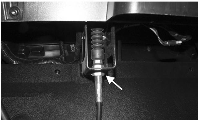
4. Remove the E-clip securing the cable end to the shift arm stud.
