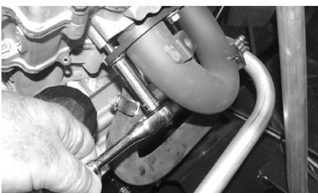
14. Disconnect the O2 sensor; then remove the O2 sensor.
