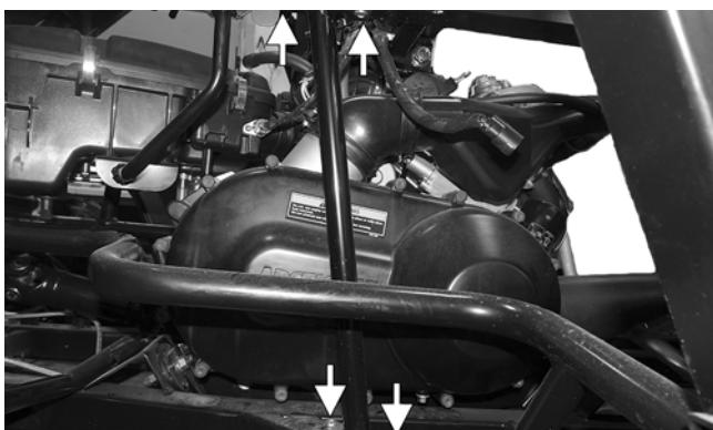
5. Remove the cap screws securing the CVT cover noting the location of the different-lengthed cap screws for installing purposes; then using a rubber mallet, gently tap on the cover tabs to loosen the cover. Remove the cover.
