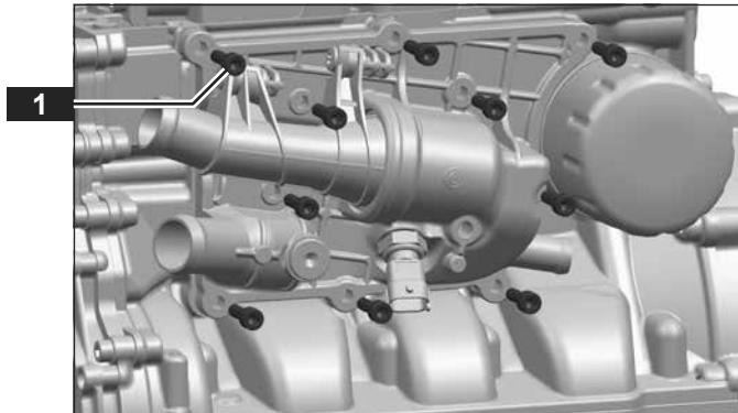
The thermostat housing is caulked with a silicone liquid seal.
