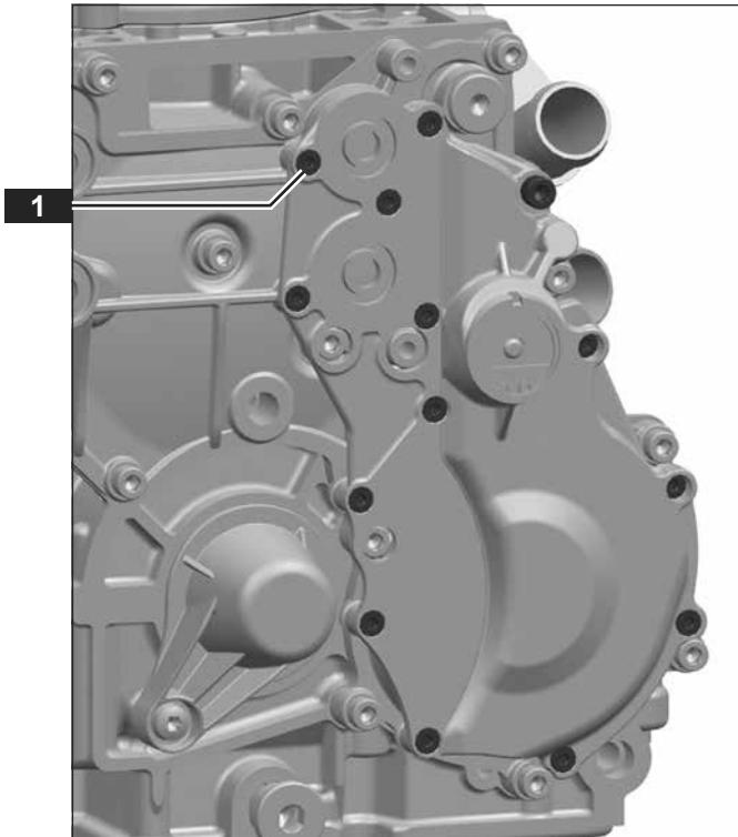
The cover oil cooler bracket is caulked with a silicone liquid seal.
