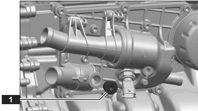
**050.01.08 Removing closing cap thermostat housing**
