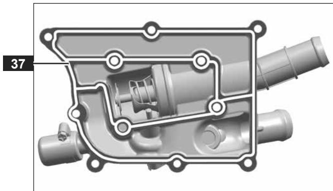
► Hold the thermostat housing **38** in position.
