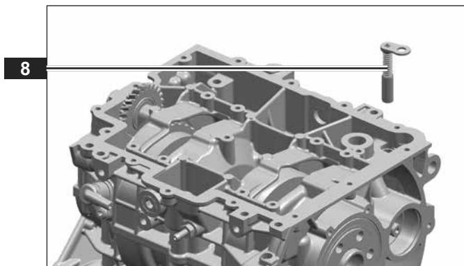
The crankcase is caulked with a silicone liquid seal.
