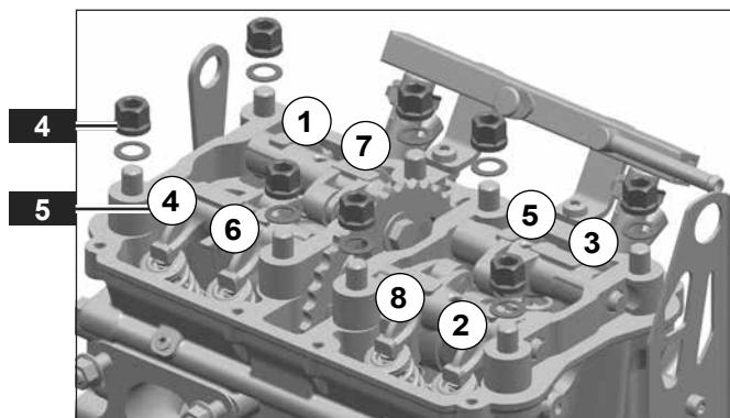
► Remove the cylinder head **6**.
