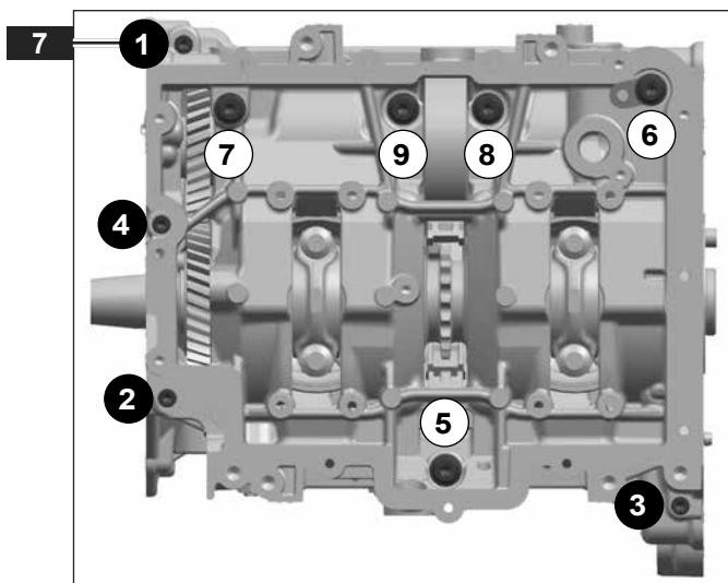
► Pull the oil pressure valve **8** out using a bar magnet.
