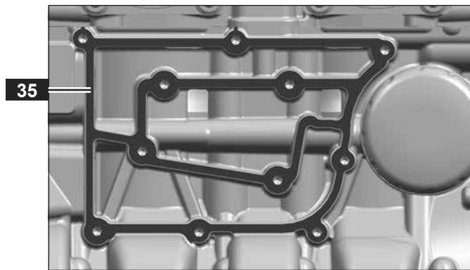
► Clean the sealing surface **36** with sealing surface cleaner.
