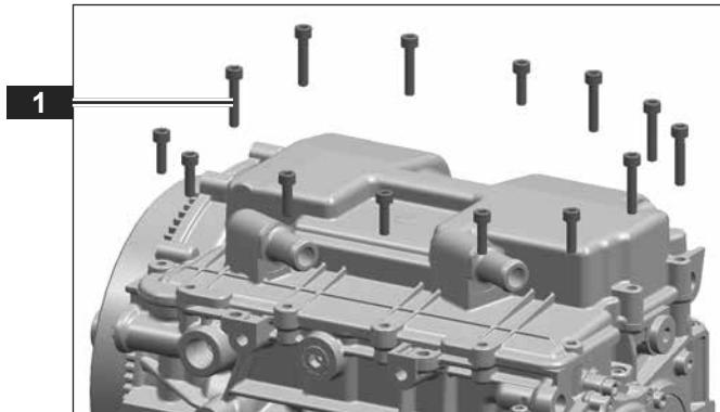
The suction pump cover is caulked with a silicone liquid seal.
