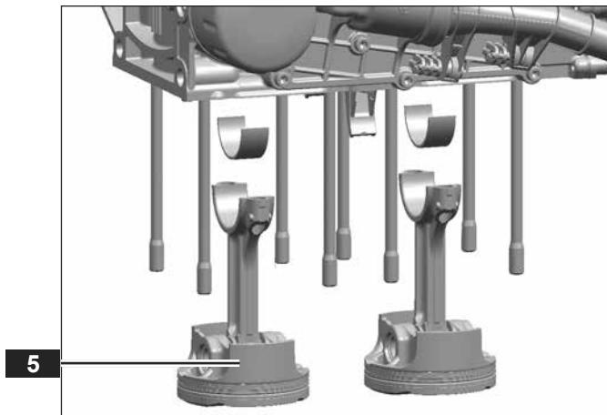
**020.01.06 Installing pistons and con rods**
