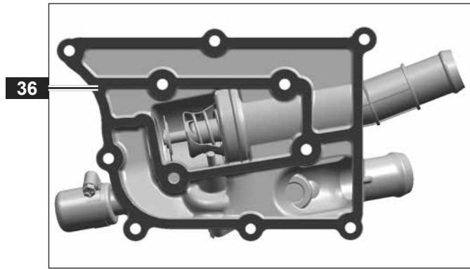
► Apply the silicone liquid seal **37** without gaps as illustrated.
