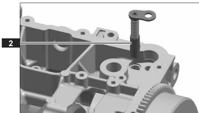
**110.03.02 Installing oil pressure valve**
