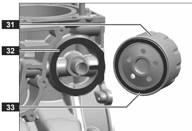
► Screw in the oil filter **34** by hand.
