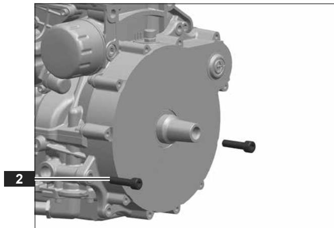
The generator cover is caulked with a silicone liquid seal.
