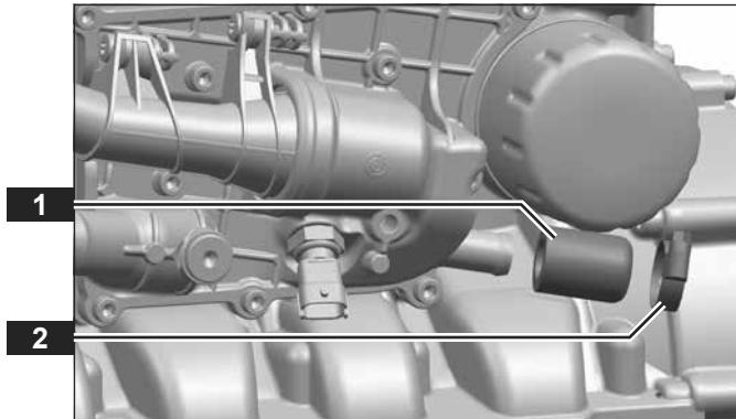
**050.01.09 Installing closing cap thermostat housing**
