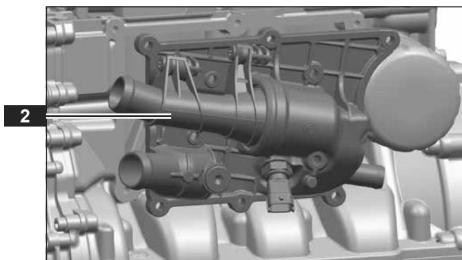
**050.01.02 Installing thermostat housing**
