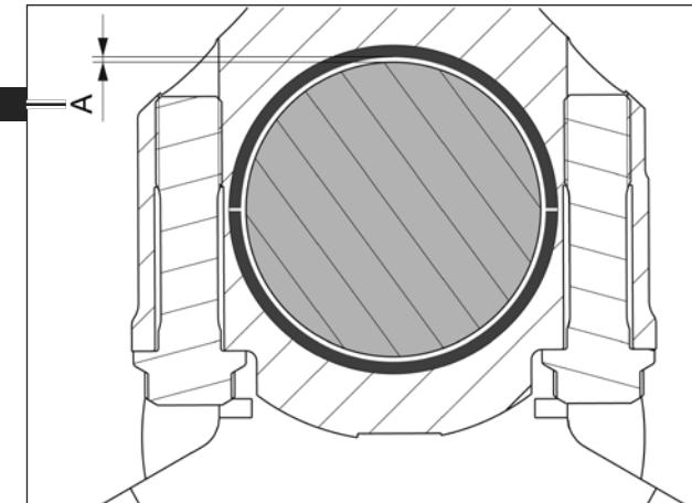
The con rod bearing shells are marked on the side **9** in color. Each color represent a specific thickness of the con rod bearing shell.
