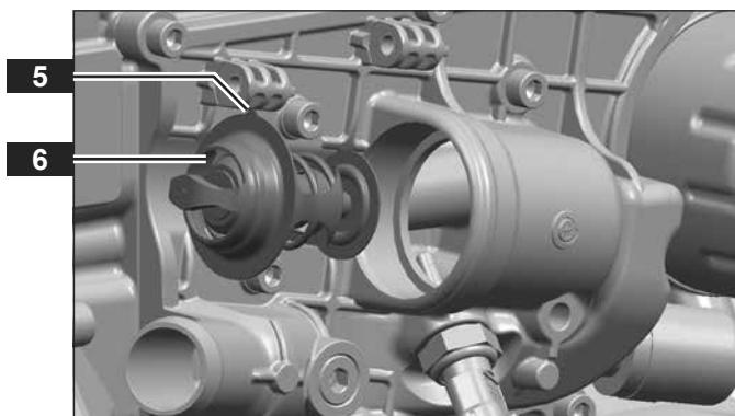
**050.01.06 Replacing sensor coolant temperature**
