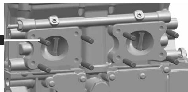
**070.01.01 Removing intake manifold**
