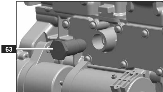
Checking the alignment of the balance shaft / crankshaft
