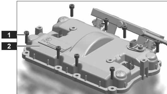
030.01.02 Installing valve cover
