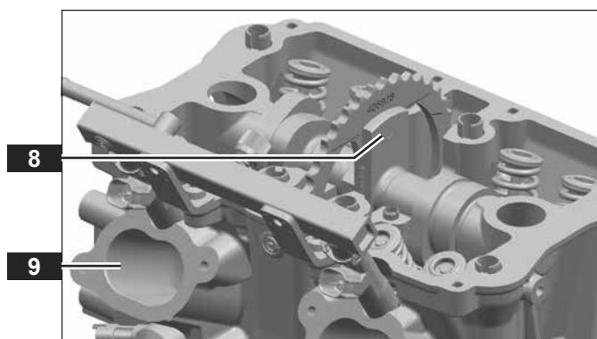
**NOTICE!** Bearing damage due to the bearing cap being installed incorrectly. The bearing surfaces for supporting the camshaft in the cylinder head and in the bearing cap are processed together. Therefore, only use the bearing cap originally installed.
