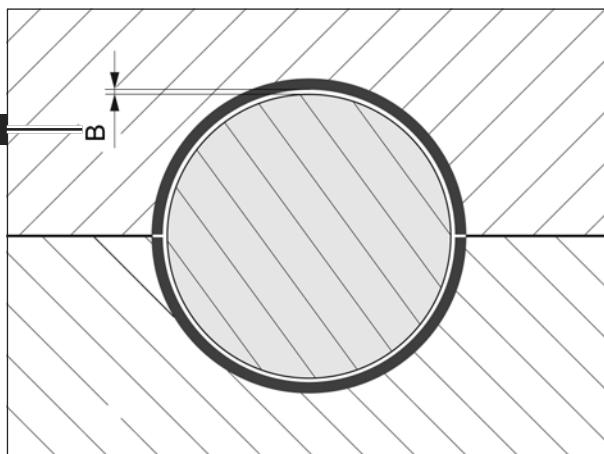
The main bearing shells are marked on the side **26** in color. Each color represent a specific thickness of the main bearing shells.
