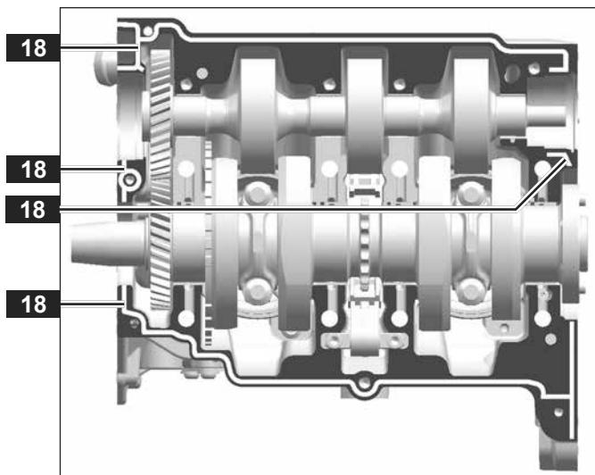
Checking the alignment of the balance shaft / crankshaft
