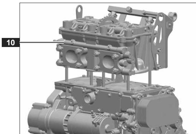
**030.02.02 Installing cylinder head**
