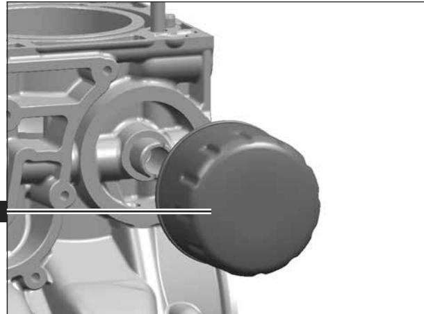
► Clean the sealing surface **35** with sealing surface cleaner.
