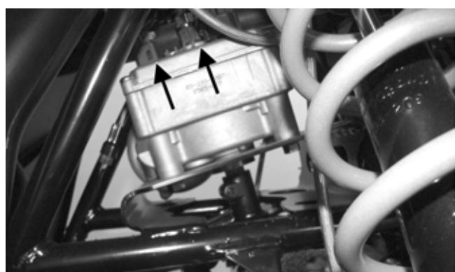
5. Align and engage the upper steering post couple to the top of the EPS unit.
