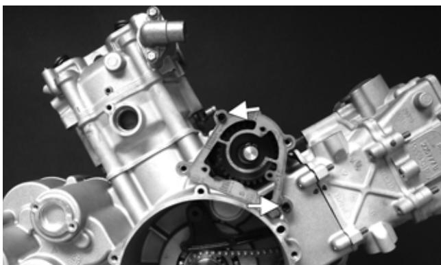
15. Remove the water pump driveshaft and gear assembly from the engine.
