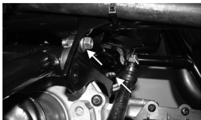
4. Remove the two cap screws and nuts securing the front differential to the frame. Account for the washers and their location.
