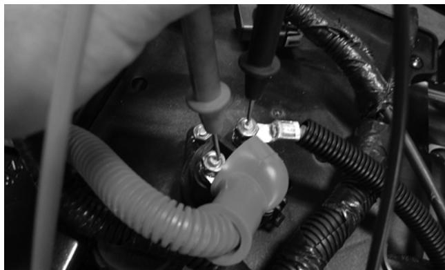
■**NOTE:** Make sure that the ignition switch is in the ON position, transmission in neutral, brake lock released, and the engine stop switch in the RUN position.
