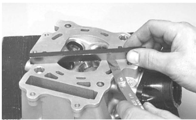
2. Inspect the cylinder for pitting, scoring, scuffing, warpage, and corrosion. If marks are found, repair the surface using a cylinder hone (see Inspecting Cylinder in this sub-section).
