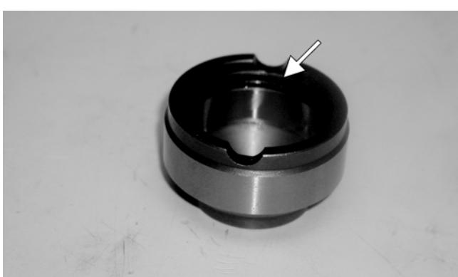
9. Apply grease to the outer edges of the clutch housing; then from inside the clutch cover, install the clutch housing into the cover using a rubber mallet.
