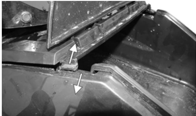
2. Release the front storage tray by lightly squeezing the left and right outside edges inward.
