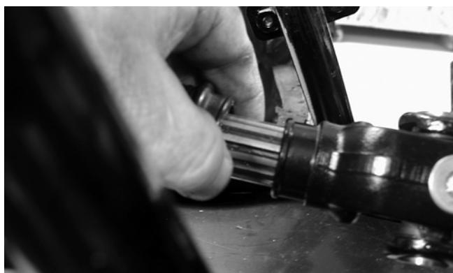
3. Install the two through-bolts. Secure with lock nuts and tighten to 35 ft-lb. Tighten the rear drive flanges to 20 ft-lb; then tighten the rear gear case through-bolts to 35 ft-lb.
