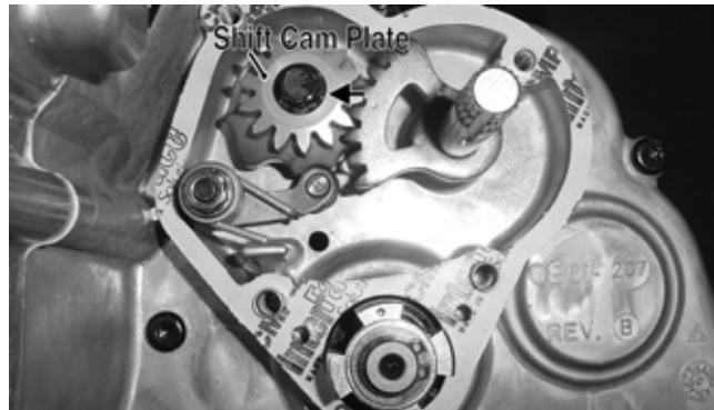
13. Remove the snap ring securing the speed sensor trigger to the shaft. Remove the thrust washer; then remove the trigger using a suitable “two-jawed” puller. Account for a gasket.
