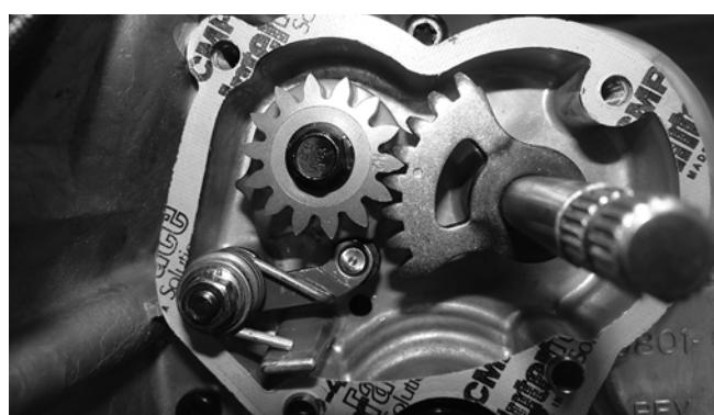
8. Apply grease to the lips of the shift shaft seal in the gear shift cover. Install the dowel pins; then using a new gasket, install the gear shift cover and secure with the cap screws. Tighten in a crisscross pattern to 8 ft-lb.
