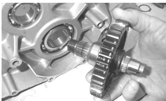
2. Install and tighten the output shaft flange nut to 59 ft-lb. Using a punch, peen the nut.
