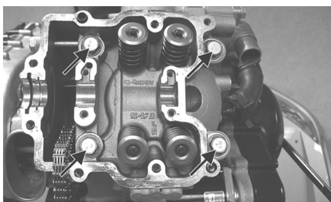
9. Loosely install the five cylinder head nuts.
