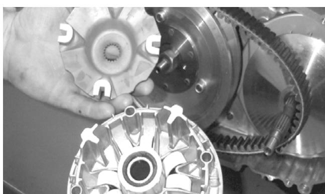
5. Using a 6 mm cap screw threaded into the fixed driven face, spread the driven pulley by turning the cap screw clockwise; then remove the V-belt.
