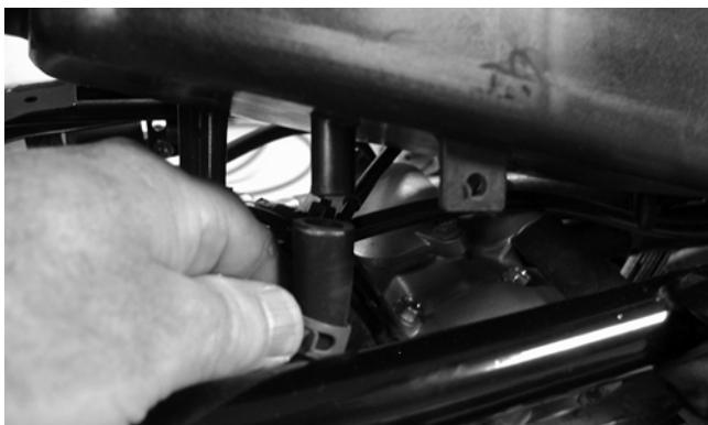
5. Remove the gasoline hose connector from the fuel rail.
