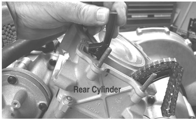
7. Place a new head gasket into position on the cylinder. Place the alignment pins into position; then place the head assembly into position on the cylinder while guiding the cam chain through the cylinder head.
