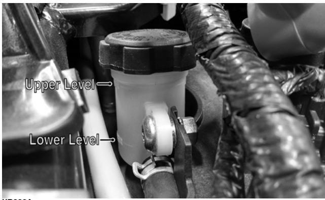
2. Compress the brake lever/pedal several times to check for a firm brake. If the brake is not firm, the system must be bled.
