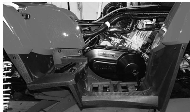
2. Remove the cap screws securing the CVT cover; then using a rubber mallet, gently tap on the cover tabs to loosen the cover. Remove the cover. Account for two dowel pins.
