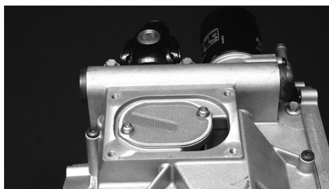
2. Remove the cap screws securing the lower crankcase to the upper crankcase halves; then using a rubber hammer, free the lower crankcase and remove. Account for two alignment pins.
