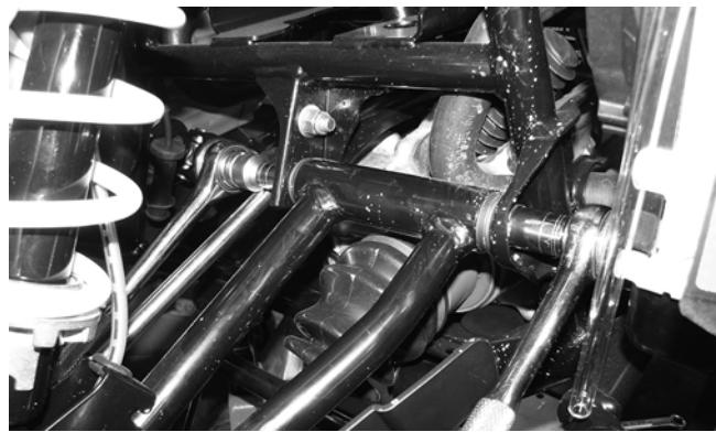
3. Remove the cap screws and lock nuts securing the A-Arm brace to the frame. Discard the lock nuts. Remove the A-Arm brace.
