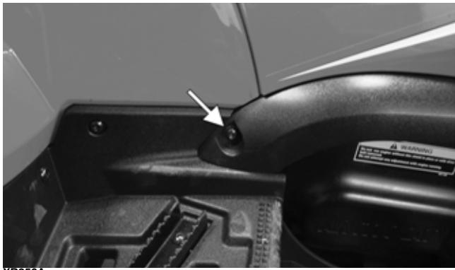
7. Remove the four lock nuts securing the front rack assembly to the frame.
