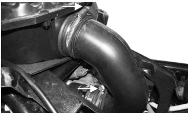
4. Disconnect the crankcase breather hose from the air filter housing; then remove the air filter housing.
