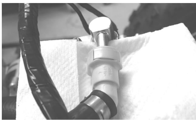
5. Disconnect the TPS (A), MAP sensor (B), and ISC valve (C) from the throttle body; then route the harness and connectors away from the engine.
