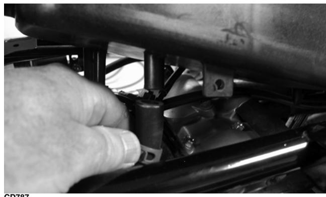
8. Remove the gasoline hose connector from the fuel rail.
