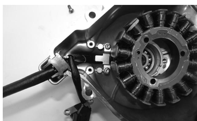
3. Install the new stator coil assembly and secure with three cap screws using a drop of red Loctite #271 on each. Tighten according to the chart.
