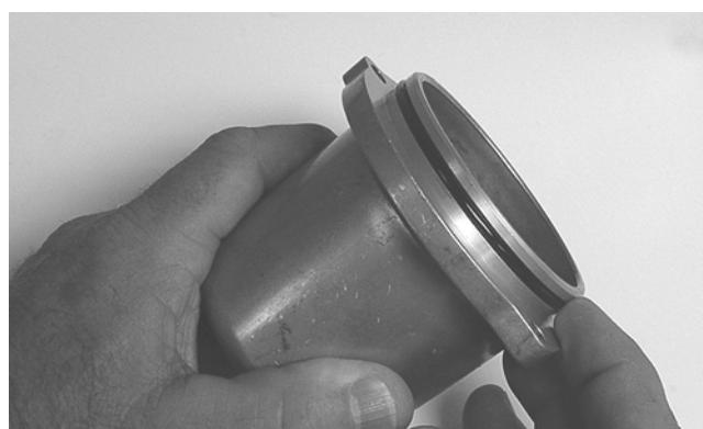
3. Clean the countershaft and trigger splines thoroughly and install the inner snap ring onto the shaft; then apply green Loctite #620 to the trigger and countershaft splines and install the trigger. Secure with a flat washer and outer snap ring.
