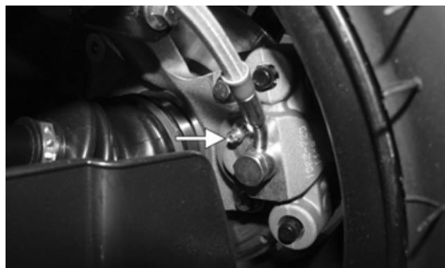
**■NOTE: During the bleeding procedure, watch the reservoir very closely to make sure there is always a sufficient amount of brake fluid. If low, refill the reservoir before the bleeding procedure is continued. Failure to maintain a sufficient amount of fluid in the reservoir will result in air in the system.**
