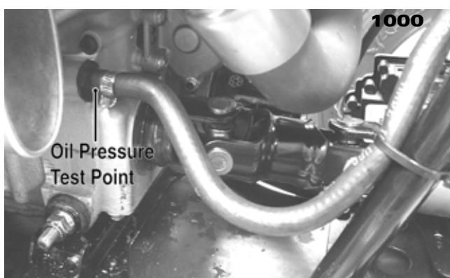
■NOTE: Some oil seepage may occur when installing the oil pressure gauge. Wipe up oil residue with a cloth.
