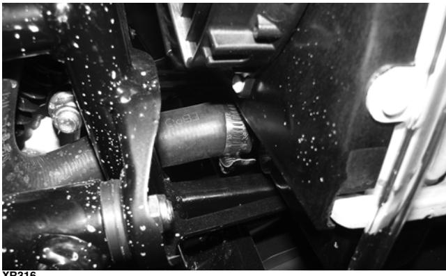
4. Fill the cooling system with the recommended amount of antifreeze (see Periodic Maintenance/Tune-up). Check for leakage.
