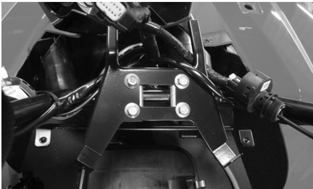
5. Remove the steel ring around the harness; then remove the two cap screws securing the upper steering post bushings to the frame. Account for two housings and steering post rear bracket.
