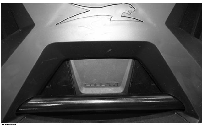
2. Carefully rotate the radiator cap counterclockwise to release pressure; then remove the cap.
