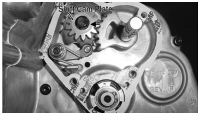
7. Install the shift shaft into the crankcase making sure the washer is properly located; then align the timing reference marks and completely seat the shift shaft.
