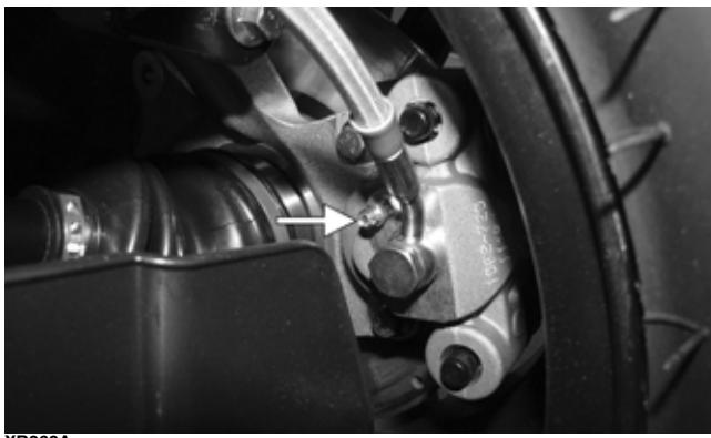
**■NOTE: During the bleeding procedure, watch the sight glass very closely to make sure there is always a sufficient amount of brake fluid. If low, refill the reservoir before the bleeding procedure is continued. Failure to maintain a sufficient amount of fluid in the reservoir will result in air in the system.**
