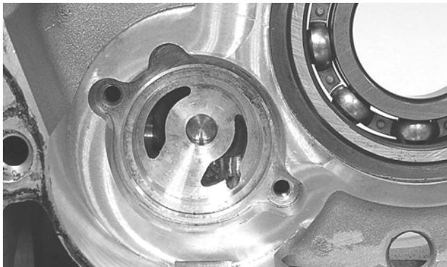
3. Inspect the gerotor set for scoring, discoloration, or cracks; then using a feeler gauge, check the inner to outer rotor clearance. If measurements exceed specifications, the gerotor set must be replaced.
