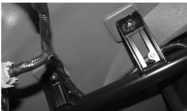
8. Remove the two self-tapping screws securing the front grille and the two cap screws located behind the grille securing the front fascia to the bumper frame.
