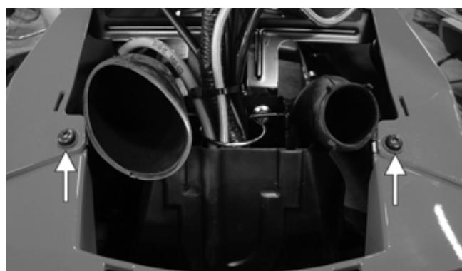
5. From the left side, remove the shift lever knob and the remaining reinstallable rivet to remove the left side panel.
