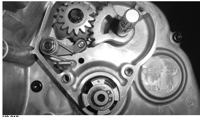
6. Install the shift cam plate onto the shift cam shaft and secure with the cap screw. Tighten to 8 ft-lb.
