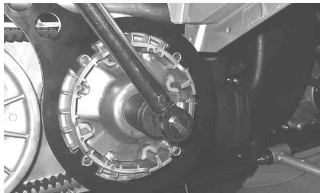
■NOTE: At this point, the cap screw can be removed from between the driven clutch faces.
