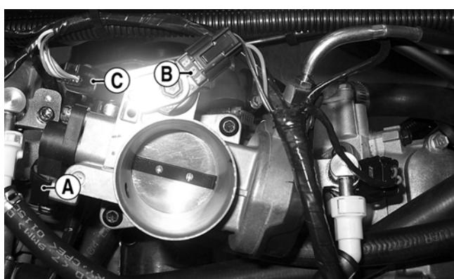
6. Disconnect the fuel injector wiring connectors, leaving the injectors installed.
