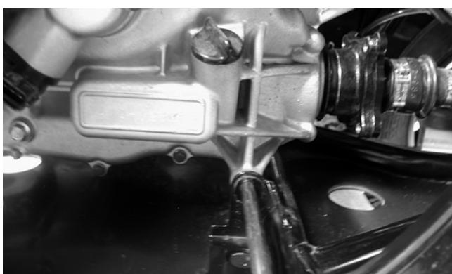
25. Move the engine to the rear enough to allow the front driveshaft to clear the front output yoke. Account for the spring; then move the engine forward and to the left. The engine will come out the left side of the frame.
