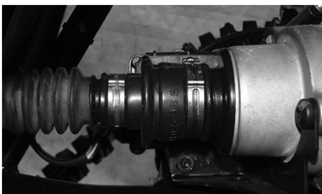
19. Free the differential assembly from the frame; then shift the differential assembly forward enough to disengage the front driveshaft from the output yoke.
