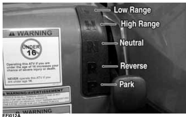
Stop the ATV completely and shift the transmission into the R position.
