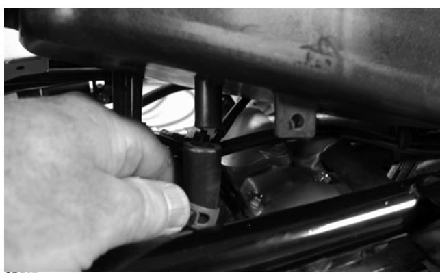
12. Remove the fuel hose connector from the fuel rail.
