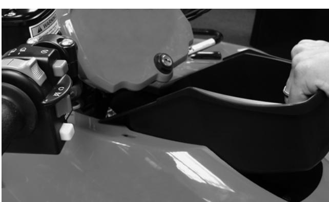
6. Remove the four cap screws securing the handlebar caps and indicator display bracket to the steering post; then move the handlebar and gauge out of the way. Account for four handlebar caps.
