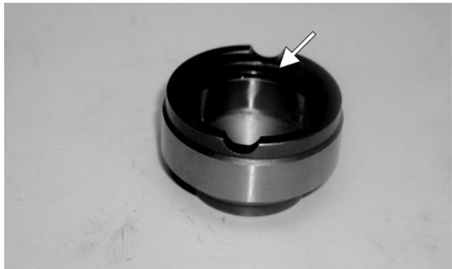
8. Apply grease to the outer edges of the clutch housing; then from inside the clutch cover, install the clutch housing into the cover using a rubber mallet.
