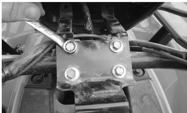
7. Remove two cap screws securing the upper steering post bearing to the frame. Account for two steering post mounting blocks and steering post mounting bracket.
