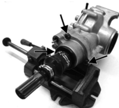
2. Using a rubber mallet, remove the housing. Account for a gasket. Remove the fork, collar, and spring. Note the location of all the components for assembling purposes.
