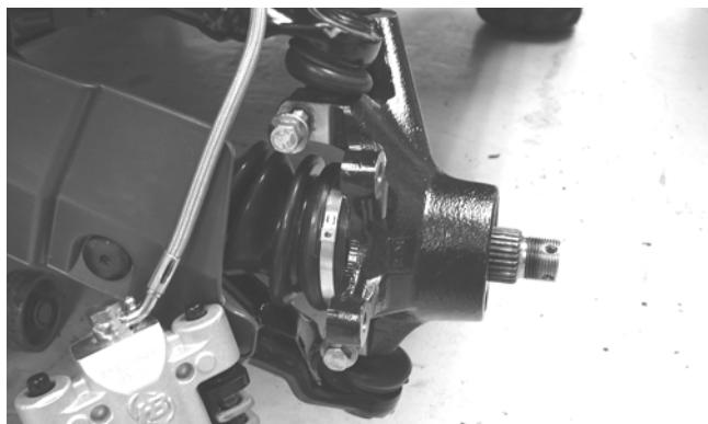
8. Tap the ball joints out of the knuckle; then remove the knuckle.
