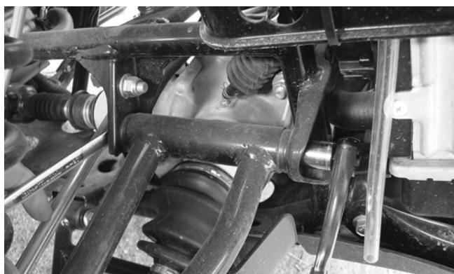
15. Push the axle shaft firmly toward the differential to release the internal lock; then while holding the axle in, pull the CV cup from the differential.
