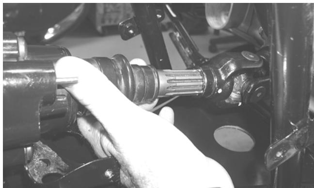
20. Place the differential on its right side; then remove it from the frame.
