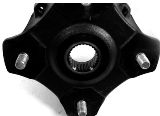
4. Secure the hub assembly with the hex nut. Tighten only until snug.
