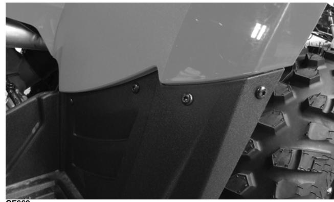
2. Remove the screws and flange nuts securing the foot pegs to the footrests; then remove the foot pegs and footwells.
