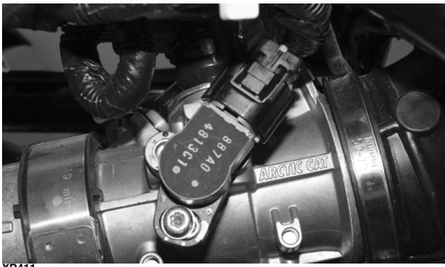
■**NOTE:** Prior to testing the TPS, inspect the three-wire plug connector on the main harness and the three-pin plug on the TPS for contamination, broken pins, and/or corrosion.
