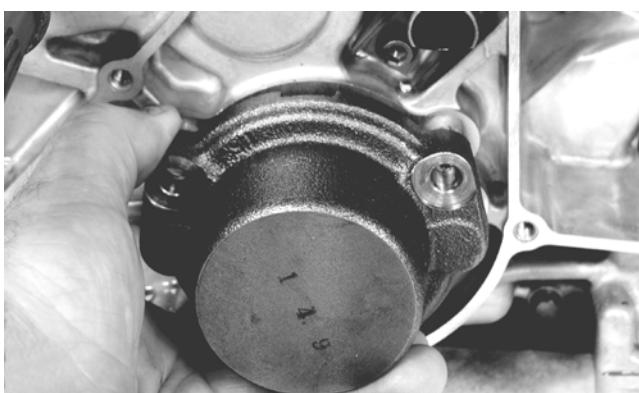
13. Remove the snap ring securing the oil pump driven gear (A); then remove the gear noting the direction of the sides of the gear for installing purposes. Account for a pin and a washer.
