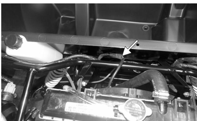
3. Remove the two shoulder bolts and nuts securing the radiator to the frame; then disconnect the upper and lower coolant hoses. Remove the reservoir tank hose from the radiator filter neck.
