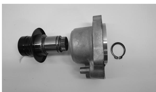
3. Using an appropriate seal puller, remove the seal from the front of the housing.
