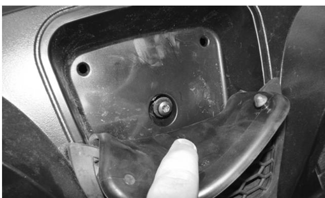
2. Secure the tilt steering sub-assembly to the support lift with the cap screw and new lock nut. Connect the headlight switch connector; then install the steel access panel with two cap screws.
