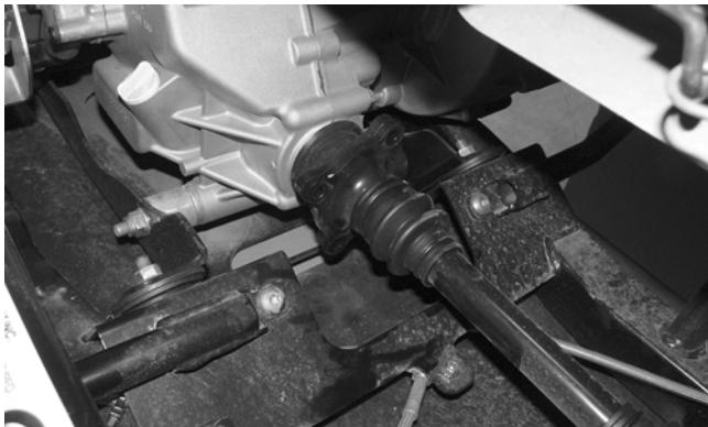
19. Remove the cap screws and lock nuts securing both left- and right-hand frame braces to the frame.
