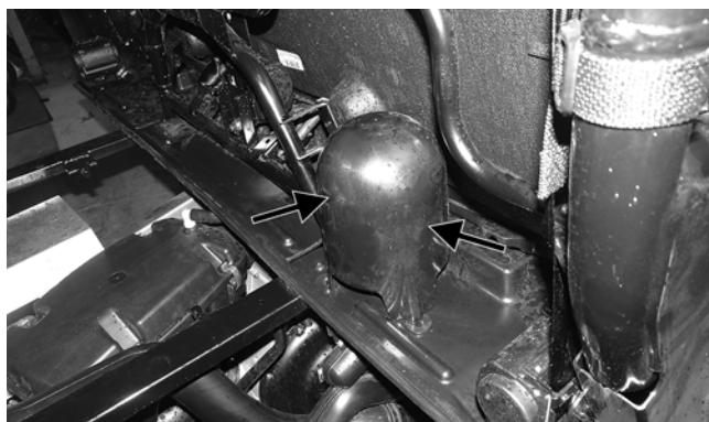
2. Loosen the clamp securing the pre-filter.
