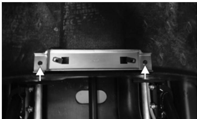
3. Place the front of the center footrest into position in the vehicle first; then lower the rear.
