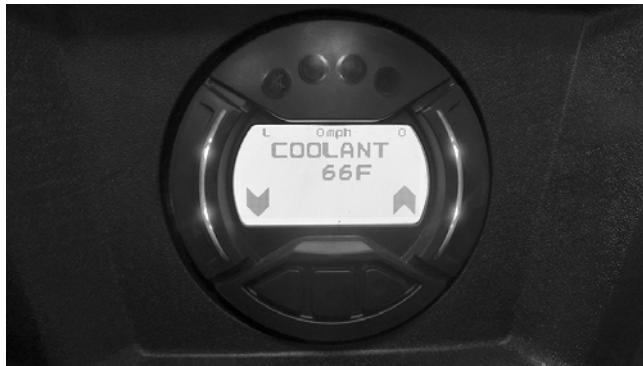
Display: Engine coolant temperature as measured by the ECT sensor.
