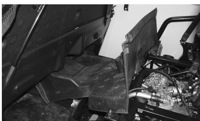
4. Secure the center footrest to the support bracket and frame.
