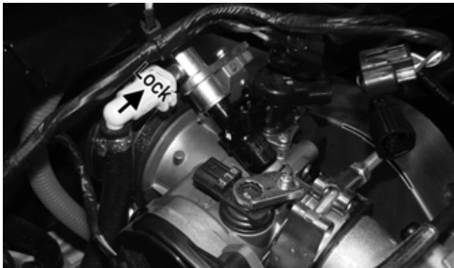
19. Connect the MAP sensor connector (A), fuel injector connector (B), ISC connector (C), and TPS connector (D); then install new nylon ties as noted during removing.
