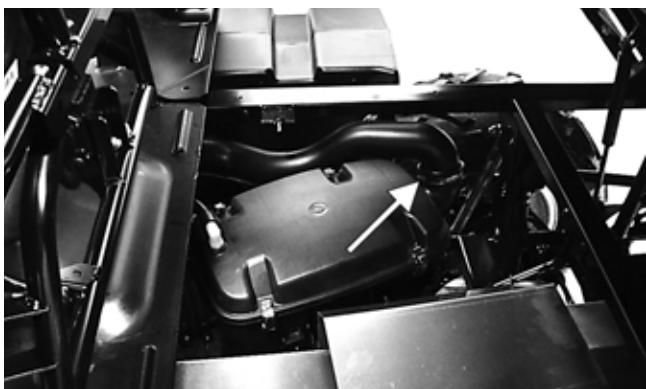
7. Remove the cap screws securing the air filter to the frame; then loosen the air inlet boot clamp and disconnect the IAT sensor connector and remove the air filter assembly.
