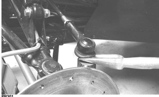
3. Remove the EPS unit and cradle bracket; then remove the cap screws securing the steering rack assembly to the rack bracket and remove from the left side.
