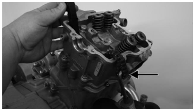
10. Remove the five nuts securing the cylinder head to the cylinder.
