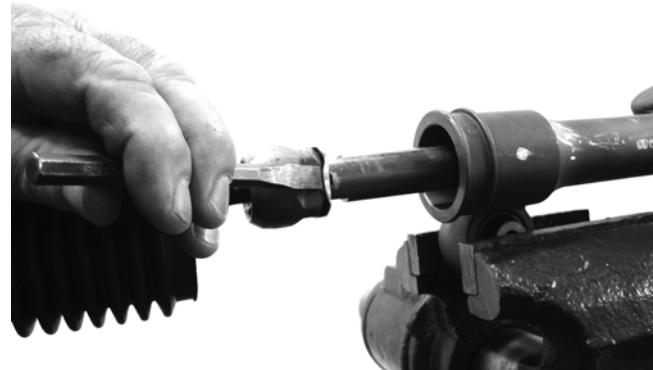
4. Using an appropriate crow-foot and backing wrench, remove the tie rod assembly.
