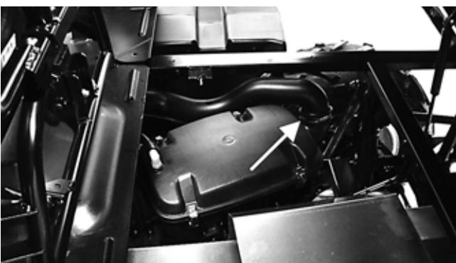
18. Connect the gasoline hose to the throttle body making sure the gasoline hose connector fully engages and locks onto the fuel rail.
