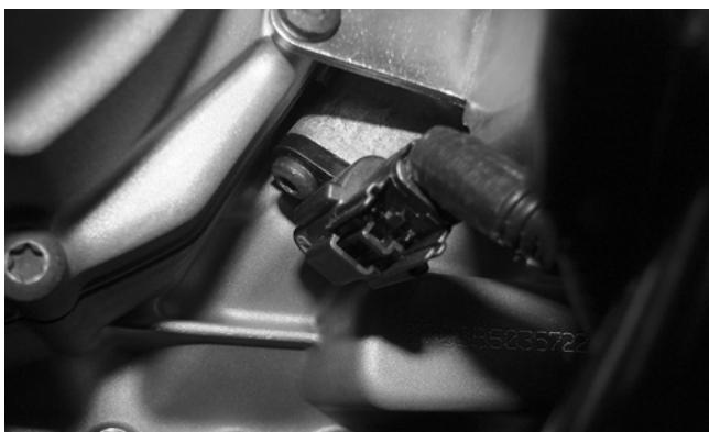
10. Remove the cap screws securing the shift cable bracket to the engine case. Remove the cap screw from the shift arm and disconnect the gear position switch connector. Slide the gear position switch off the engine.
