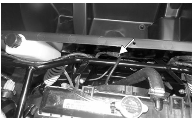
4. Open the high-point bleed screw on the top of the thermostat cover (located under the rear seat base) to allow trapped air to escape. Tighten securely after filling.
