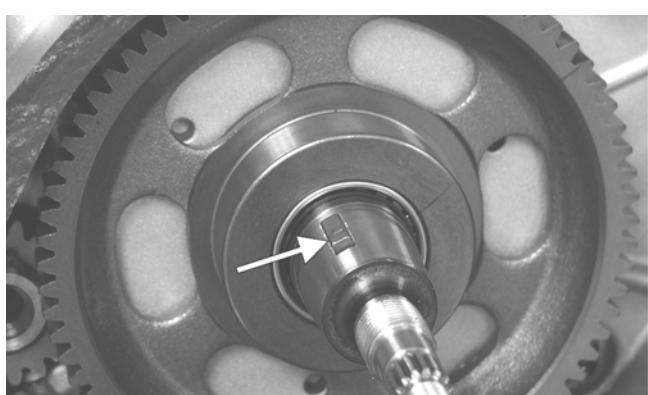
10. Remove the two starter gears from the crankcase noting the direction of the beveled side of the starter idler gear #2 for installing purposes; then remove the two starter gear shafts.
