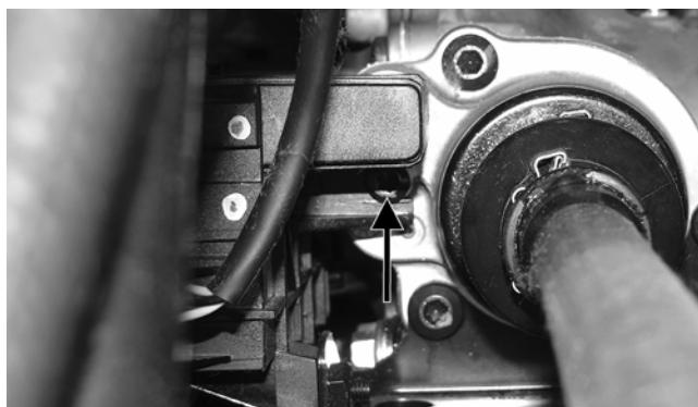
3. Remove the mounting cap screw from below the actuator on the suspension side.
