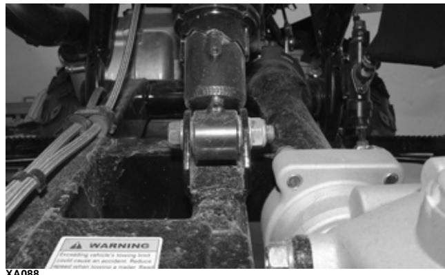
**■NOTE: Support the swing arm with a block of wood or other support to allow removal of the cap screw.**
