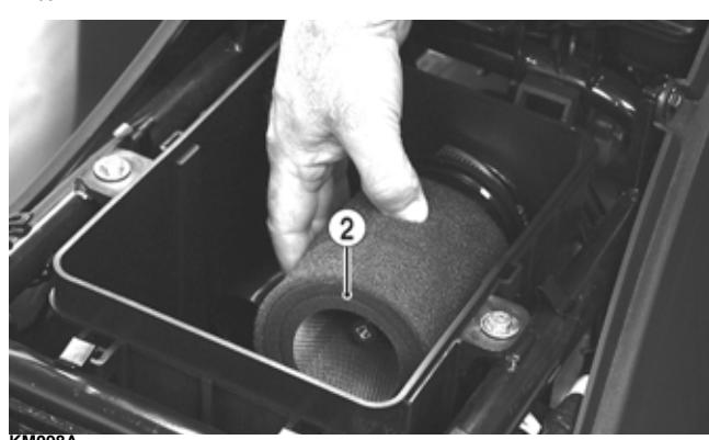
4. Place the elements in a pan larger than each element and spray generously with cleaning solvent. Let sit approximately three minutes.
