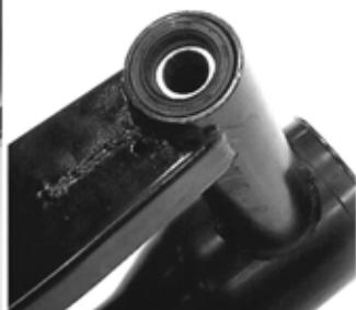
6. Align the swing arm assembly in the frame and engage the universal joint onto the splines of the secondary driven bevel gear shaft.
