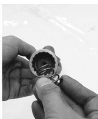
**■NOTE: Apply a liberal amount of grease to the driveshaft splines and the driveshaft spring. This will aid in keeping the spring in position while assembling.**
