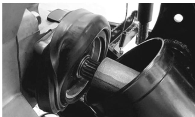
7. Install the right pivot bolt and left pivot adjusting bolt and tighten securely; then move the swing arm up and down to seat the bearings. Tighten the left pivot bolt to 36 in.-lb and the right pivot bolt to 82 ft-lb.
