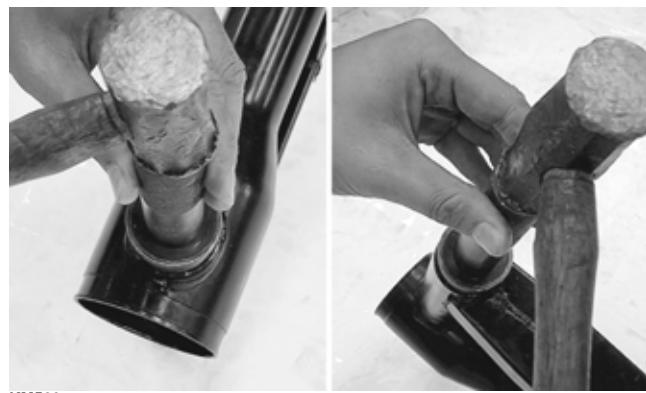
3. Remove the three cap screws, the dust plate, and one O-ring from the left axle housing on the swing arm; then from the right side, drive out the axle bearing.
