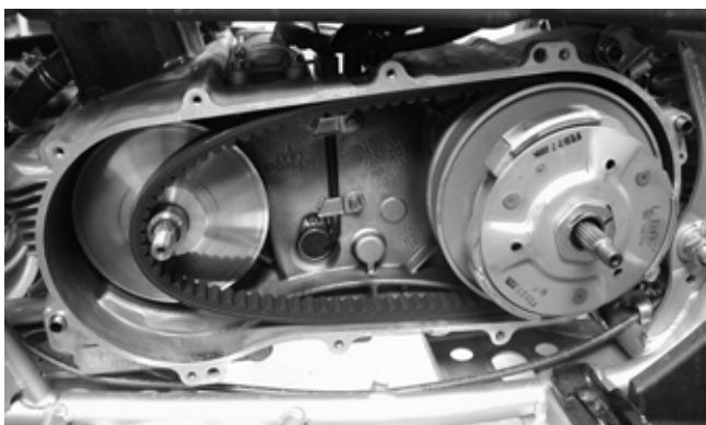
5. Remove the nut securing the driven pulley; then remove the splined bushing, centrifugal clutch, pulley, and V-belt.
