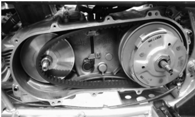
3. Install the movable drive face onto the crankshaft making sure to “bottom” the sheave out against the center bushing. The crankshaft splines should be visible and the stepped washer should sit over the splines.
