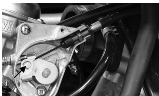
7. Loosen the outer jam nut securing the throttle cable to the carburetor body; then route the cable out of the way.
