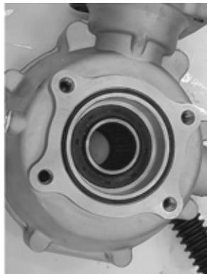
3. Inspect all splines and hubs for excessive wear, chips, cracks, or distortion.
