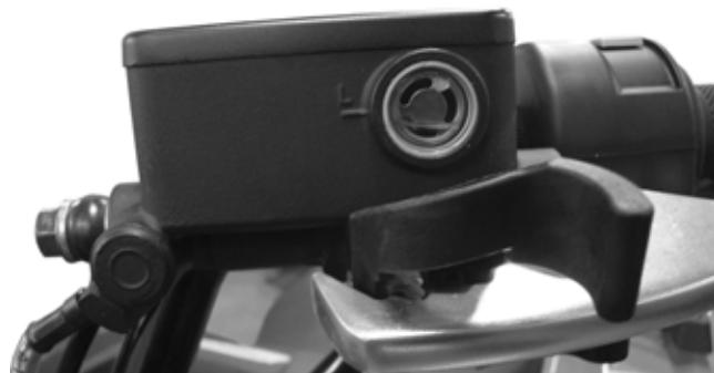
2. Compress the brake lever/pedal several times to check for a firm brake. If the brake is not firm, the system must be bled.
