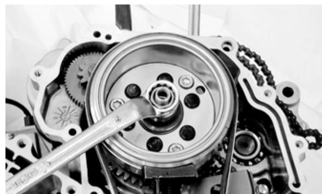
18. Install the flywheel puller and crankshaft protector; then remove the rotor/flywheel. Account for a key and the starter one-way clutch bearing.
