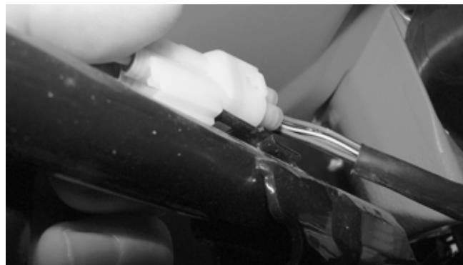
4. Secure the front body panel to the gas tank; then install both footwells.
