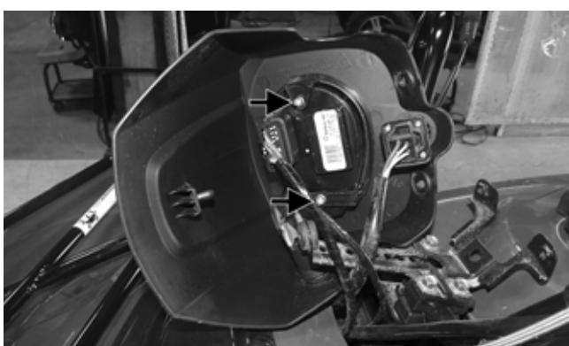
3. Install the new gauge and mounting bracket; then connect the wiring harness to the gauge.
