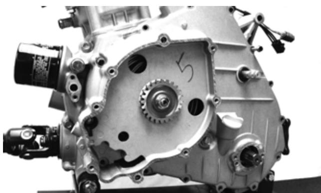
11. Install two alignment pins and a gasket on the magneto cover; then install the water pump housing assembly. Tighten the cap screws to 8 ft-lb.
