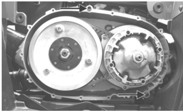
3. Mark the movable drive face and the fixed drive face for installing purposes; then remove the nut holding the movable drive face onto the crankshaft.
