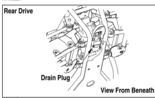
3. After all the oil has been drained, install the drain plugs and tighten to 45 in.-lb.
