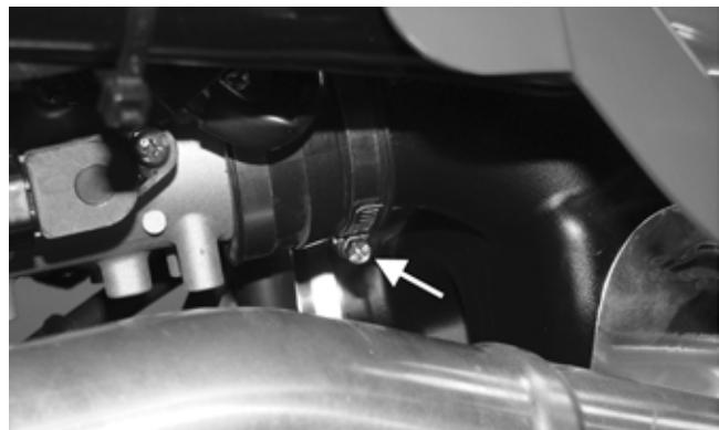
9. Disconnect the crankcase breather hose from the air intake housing and remove the air intake housing assembly.
