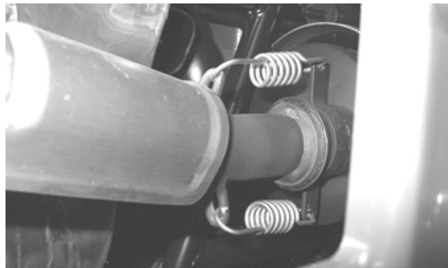
2. Slide the muffler rearward to clear the mounting lugs and remove the muffler. Account for a GRAFOIL seal.
