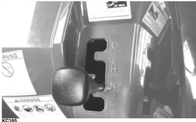
With the engine stopped and the brake lever lock engaged, turn the ignition switch to the ON position; then shift the transmission into each of the gear positions and note that the gear position indicated on the LCD corresponds to the gear position selected by the lever.
