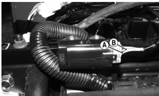
4. Tilt the sensor 60° or more to the left and right observing the meter. The meter should read 3.0-5.0 DC volts after approximately one second in the tilted position. If the meter readings are not as specified, the tilt sensor is defective.
