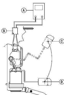
■**NOTE:** If readings are erratic, clean the resistor wiper and resistor with clean alcohol and retest. If still not correct, replace the fuel level sensor assembly.
