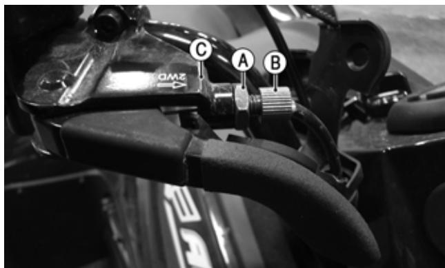
3. Remove the two cap screws securing the shift lever assembly to the handlebar.
