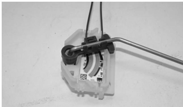
■**NOTE:** Inspect the float for any damage or leaking by submerging in water and looking for any air bubbles. Replace if damaged.
