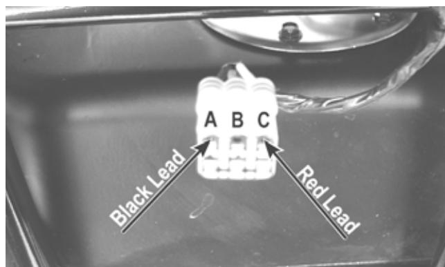
2. Turn the ignition switch to the ON position. The multimeter should read approximately 5 DC volts. If correct voltage is not indicated, check the 30-amp main and 10-amp ignition fuses, wiring harness, or the ignition switch.
