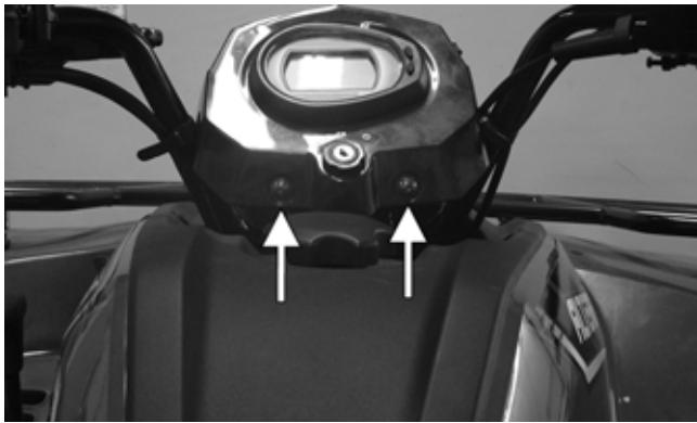
2. Unplug the gauge from the wiring harness; then remove the nuts and bracket securing the gauge to the instrument pod.
