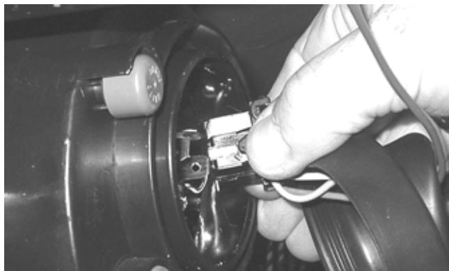
2. Press in and release the spring retainer and pull rearward clear of the bulb assembly.
