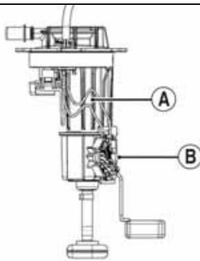
3. Keeping the float attached to the float arm, remove the float arm from the existing fuel level sensor. Press the float arm into the new fuel level sensor assembly. Ensure it locks into place.
