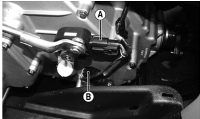
4. Drain the engine oil into a suitable container.
