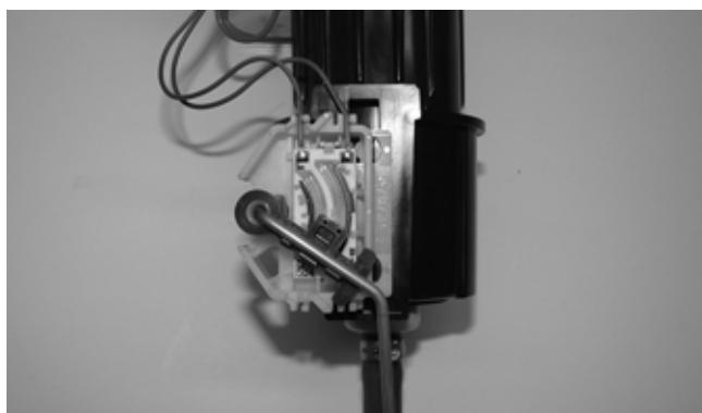
5. Shorten the wires from the fuel level sensor to approximately the same length as the previously used sensor.
