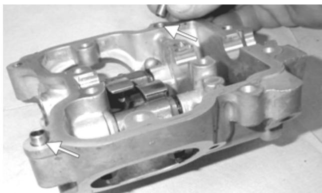
3. Remove the cap screw from the tension adjuster; then using a common screwdriver, relax the cam chain tension by rotating the adjuster screw clockwise until it locks.
