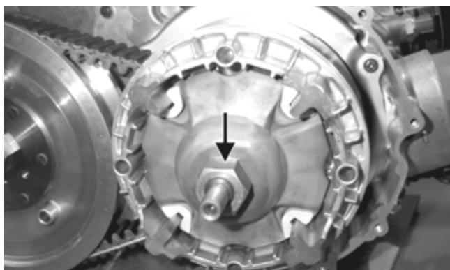
4. Remove the movable drive face and spacer. Account for the movable drive face rollers and outer drive face cover.
