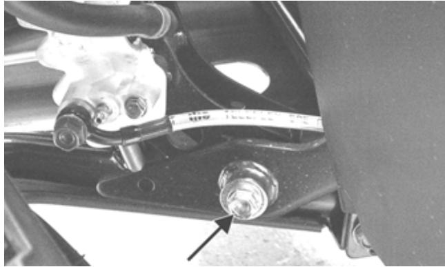
2. Remove the cap screws securing the V-belt cover to the clutch cover; then slide the brake pedal outward and remove the V-belt cover. Account for two alignment pins and a gasket.
