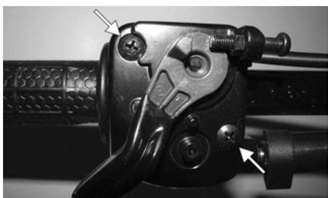
2. Slide the grommet out of the lower half of the throttle control; then remove the cable from the actuator arm.
