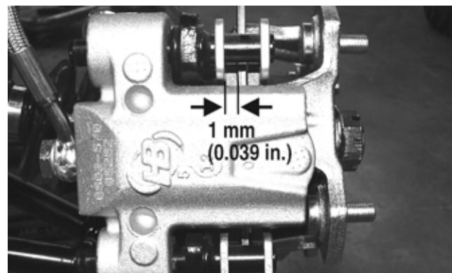
■**NOTE:** The brake pads should be replaced as a set.
