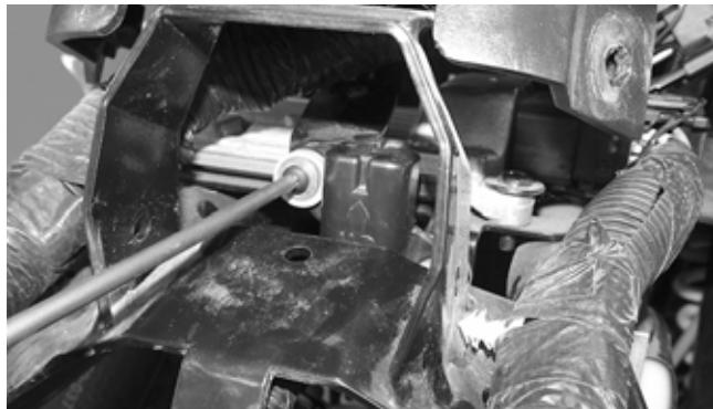
2. Install the needle adapters to the multimeter leads; then select DC Voltage on the multimeter.
