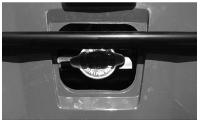
3. Add coolant as necessary; then install the radiator cap and access plug.
