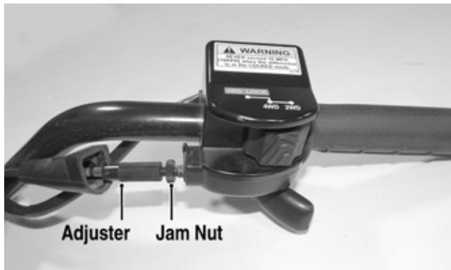
2. Turn the adjuster until the throttle cable has proper free-play of 3-6 mm (1/8-1/4 in.) at the lever.
