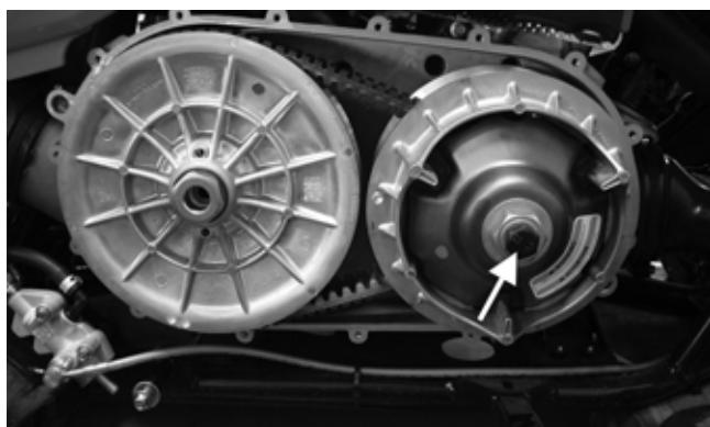
3. Using the Driven Clutch Holder to secure the driven clutch, remove the nut securing the driven assembly; then remove the driven assembly.
