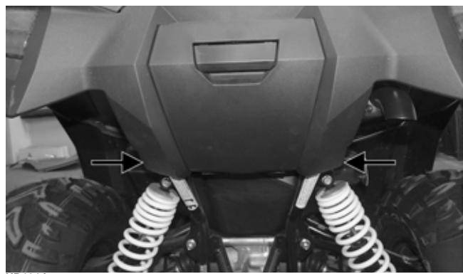
6. Remove the four lock nuts securing the rear body panel to the mounting tabs on the frame. Discard the lock nuts.
