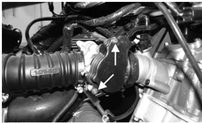
5. Remove the throttle cable from the actuator arm.
