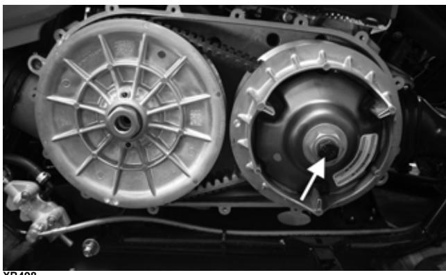
■NOTE: The arrows on the V-belt should point in the direction of rotation.
