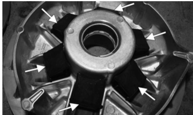
3. Check the internal bushing of the movable drive sheave. Replace as necessary. Check the fixed drive sheave internal splines for excessive wear.
