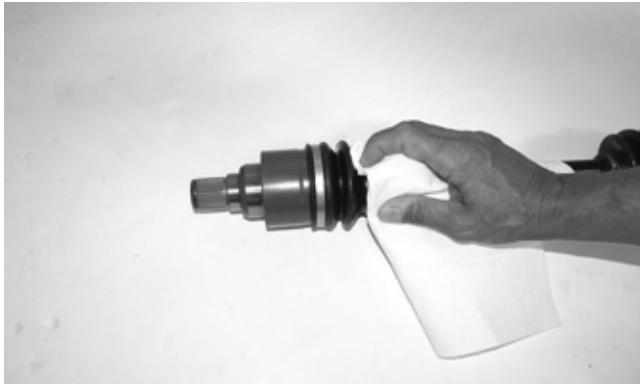
2. Inspect boots for any tears, cracks, or deterioration.
