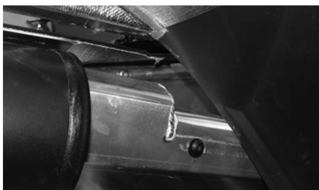
3. Slide the heat shield forward and remove the shield.
