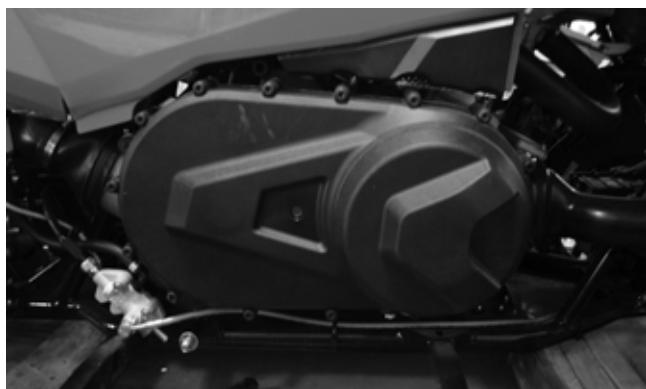
2. Remove the belt; then with the Drive Clutch Spanner Wrench to secure the drive clutch, remove the bolt securing the drive clutch; then insert the Drive Clutch Puller and remove drive clutch.
