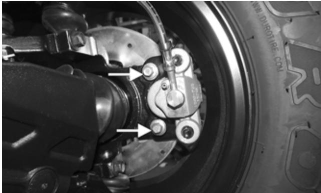
11. Tighten the hub nut (from step 9) to 200 ft-lb.
