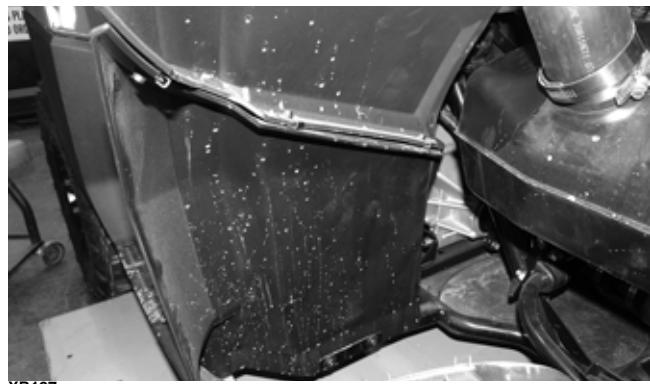
3. Remove the hose clamp securing the gas tank to the gas tank hose. Account for the hose clamp.
