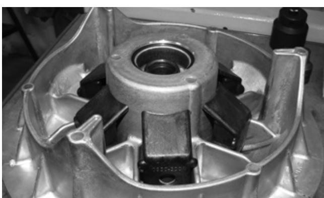
2. Note the puck orientation and locations; then remove the pucks. Check for abnormal wear. If excessively worn, replace as necessary; then remove the movable sheave from the drive clutch assembly.
