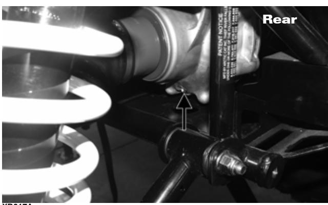
4. After all the oil has been drained, install the drain plugs and tighten securely.
