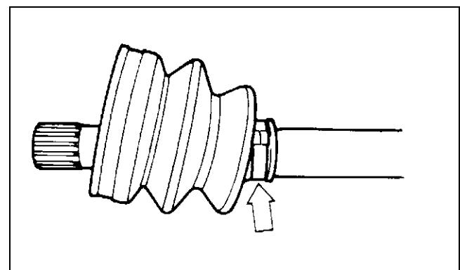
3. Apply 80 grams (2/3 of contents) of grease from the pack into the bearing housing.
