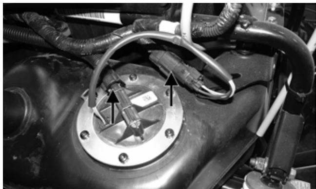
3. Remove the cable ties securing the vent hose to the frame.
