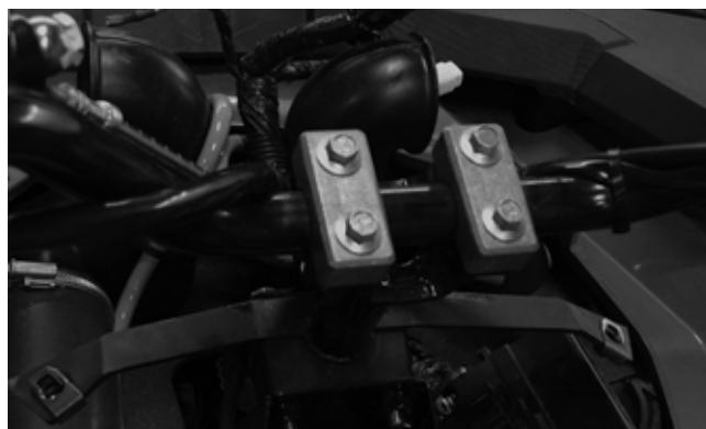
5. Remove the two cap screws securing the upper steering post housing to the frame. Account for two housings and a plate.
