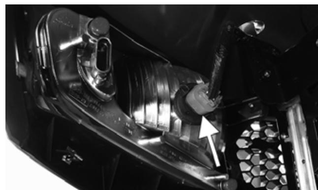
2. Connect the new headlight bulb to the wiring harness and insert into headlight assembly. Turn clockwise to secure the bulb.
