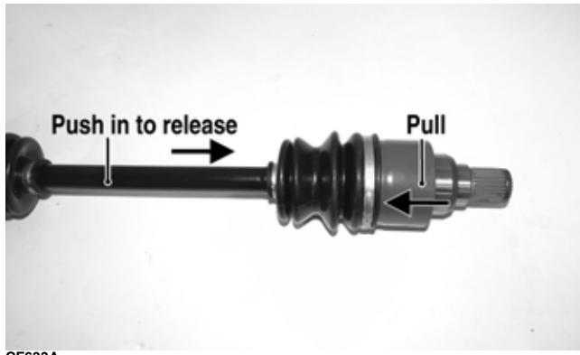
**■NOTE: To ensure proper seating of the axle, give it a light pull; the axle should remain “clipped” in place.**
