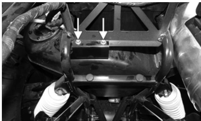
5. Remove the master cylinder from the mounting bracket; then remove the mounting bracket from the frame.
