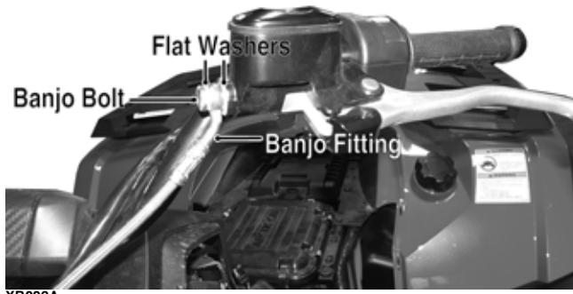
3. Install the brake lever, pivot pin, and snap ring.
