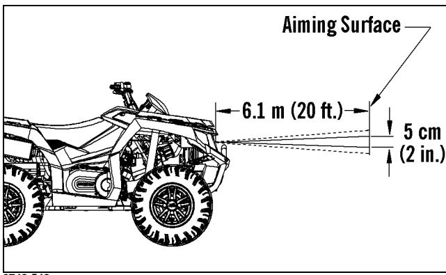
**■NOTE: There should be an average operating load on the ATV when adjusting the headlight aim.**
