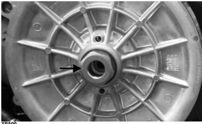
11. Spread the faces of the driven clutch by threading the cap screw from the tool kit into the boss of the driven fixed face; then tighten the cap screw until the V-belt drops into the driven pulley.
