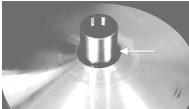
4. Install the cap screw from the tool kit into the driven pulley fixed face; then turn the cap screw clockwise to spread the pulley faces. Remove the V-belt.
