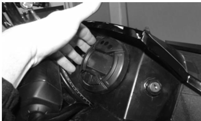
To install the gauge, connect the multi-pin connector and press the gauge into the dash.
