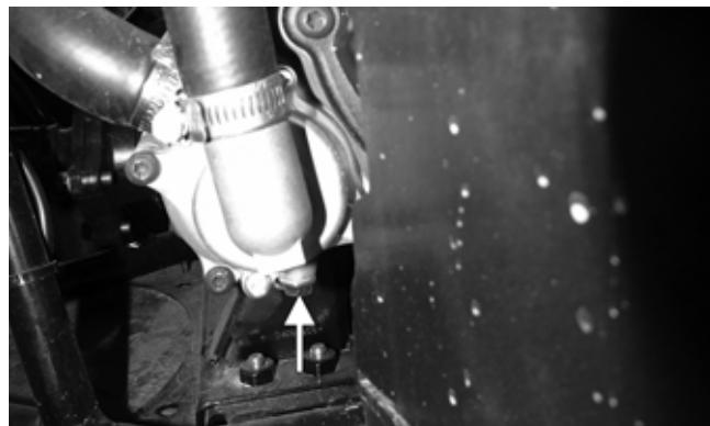
2. Drain the oil from the engine/transmission.
