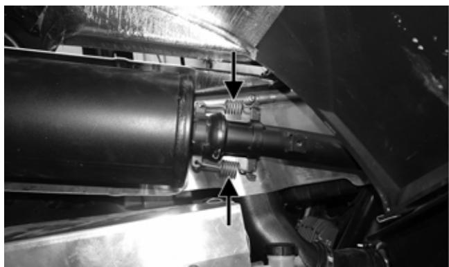
5. Remove the muffler and account for a GRAFOIL seal.
