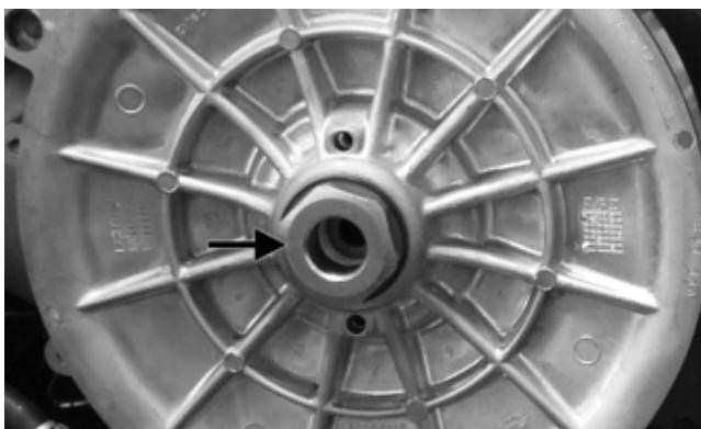
4. Remove the cap screws securing the inside clutch cover. Note the location of the different-length cap screws for installing purposes. Using a rubber mallet, carefully remove the cover. Account for two alignment pins.
