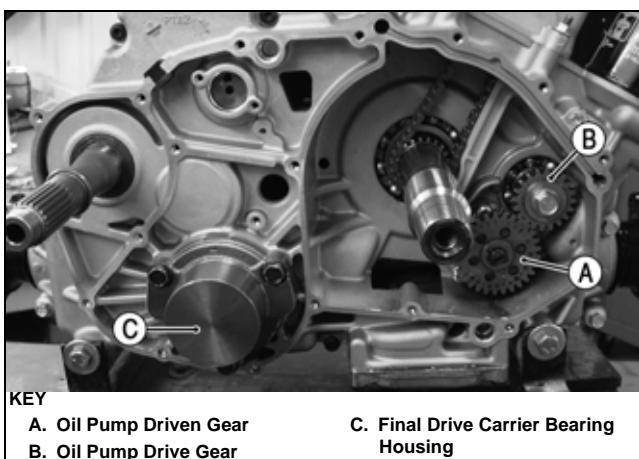
■NOTE: Account for and inspect the clutch housing seal.
