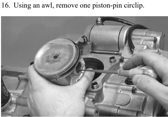
16. Using an awl, remove one piston-pin circlip.
