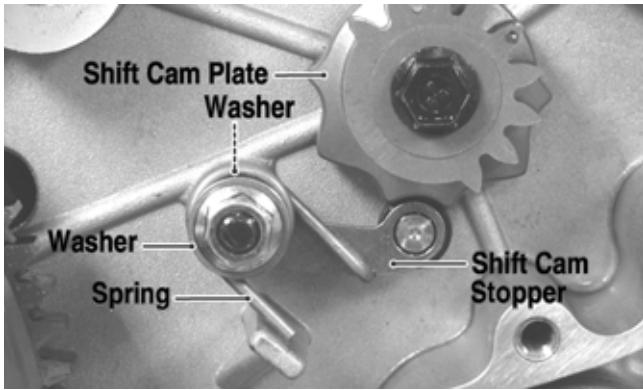
■NOTE: Rotate the shift cam plate to ensure it ratchets with no binding.
