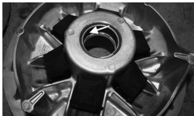
4. Remove the spring (E); then the washer (D); then the cup (C) with washer; then the plastic spacer (B); then the bearing (A). Check for any broken/excessively worn parts and replace as necessary.
