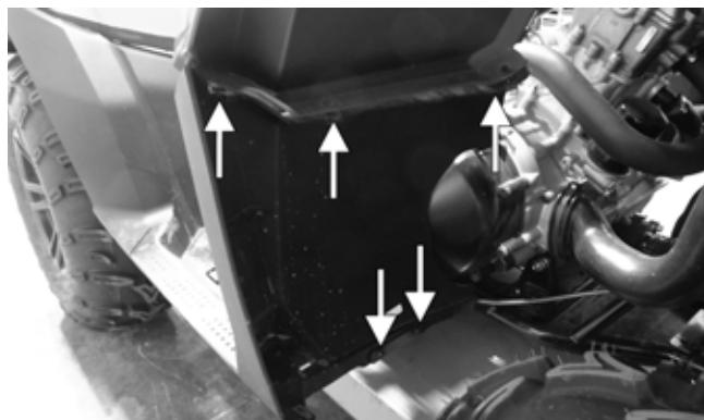
2. Remove the cap screws securing the CVT cover; then using a rubber mallet, gently tap on the cover tabs to loosen the cover. Remove the cover.
