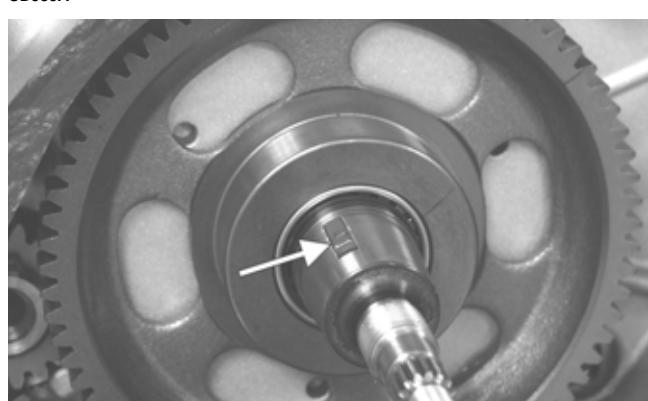
11. Remove the two starter gears from the crankcase noting the direction of the gears for installing purposes; then remove the two starter gear shafts.
