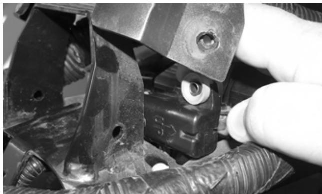
■NOTE: When replacing the sensor after testing, make sure the arrow marking is directed up.
