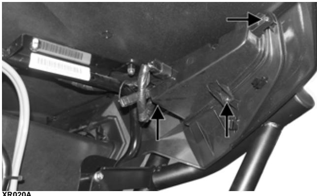
**■NOTE: The heat shield will be removed as an assembly with the right taillight.**
