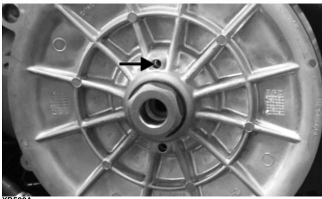
12. Place the V-belt into position on the driven pulley and then install the drive clutch onto the V-belt and crankshaft; then install and tighten the drive clutch cap screw to 59 ft-lb (80 N-m).
