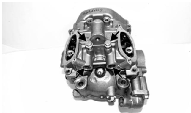
4. Remove the valve cover. Account for and note the orientation of the cylinder head plug. Note the location of the two alignment pins.
