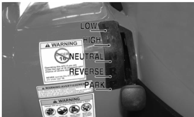
Stop the ATV completely and shift the transmission into the R position.
