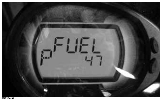
Display: Fuel level signal from the fuel level sensor (measured in ohms).
