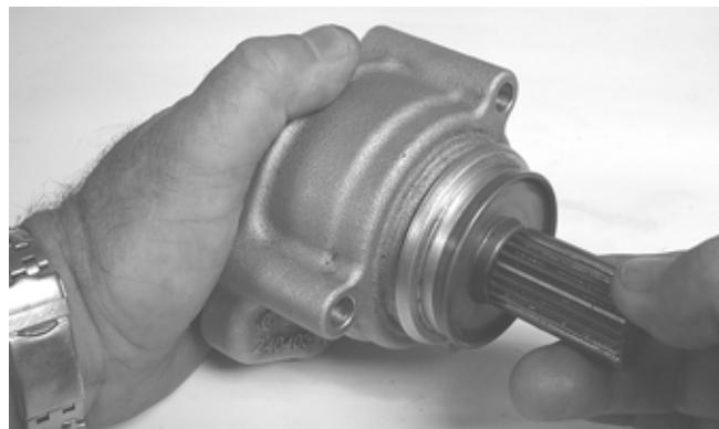
2. Remove the clutch pack from the clutch basket; then remove the snap ring securing the clutch basket (A) to the input shaft (B) and remove the clutch basket.
