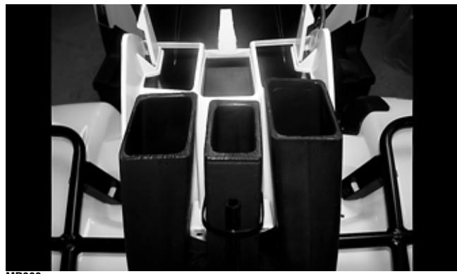
6. Remove two reinstallable rivets and remove the splash guard. The radiator cap can now be accessed in front of the snorkels.
