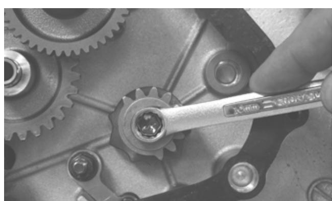
6. Install the shift cam stopper, spring, and two washers (thick washer closest to the nut); then coat the threads on the mounting stud with red Loctite #271 and install the nut. Tighten to 8 ft-lb.
