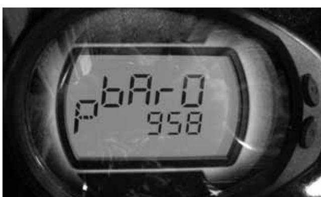
Display: MAP in millibars (958 millibar = 28.28 in. mercury).
