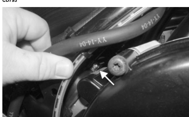
15. Remove the left-side foot peg and footwell (see Steering/Body/Controls).
