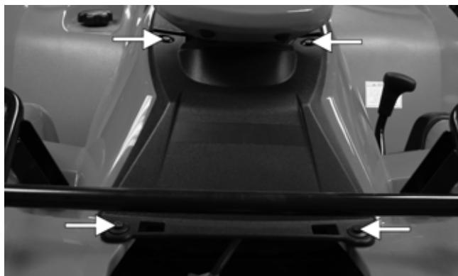
2. Unlock the storage compartment lid; then slide the storage compartment cover assembly forward and lift off the storage compartment.
