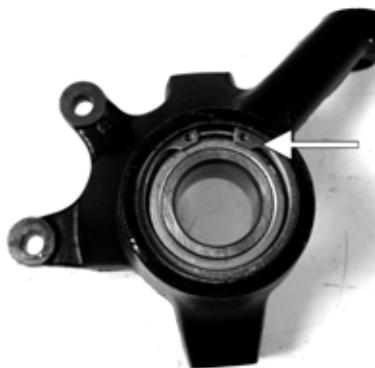
2. Install the knuckle to the upper and lower ball joints and secure with the two cap screws. Tighten to 35 ft-lb.
