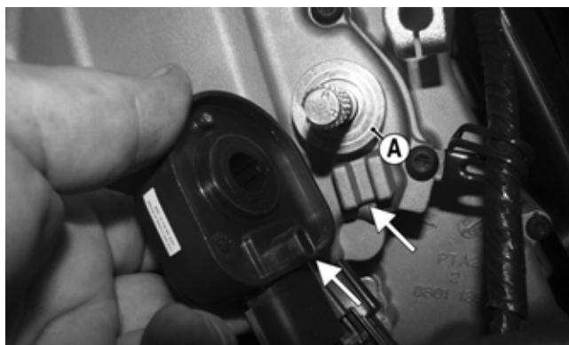
6. Remove the cap screws securing the speed sensor housing to the crankcase and remove the housing assembly; then remove the snap ring securing the speed sensor trigger and thrust washer to the shaft. Remove the trigger. Account for the gasket snap ring, and dowel pins.
