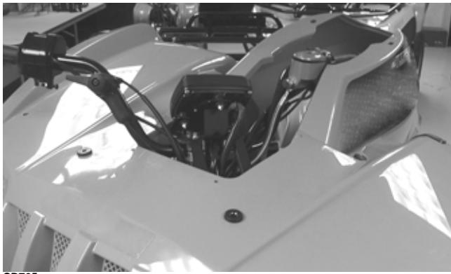
2. Connect the headlight connectors to the appropriate headlights and the front accessory plug wires to the accessory plug.
