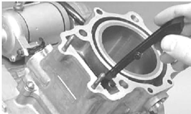
7. Place a new head gasket into position on the cylinder. Place the alignment pins into position; then place the head assembly into position on the cylinder.
