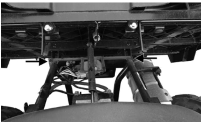
2. While an assistant holds the cargo box in the raised position, secure the end of the box lift support to the frame with the cap screw and nut.
