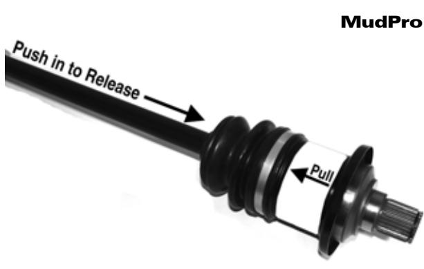
**■NOTE: To ensure proper seating of the axle, give it a light pull; the axle should remain "clipped" in place.**
