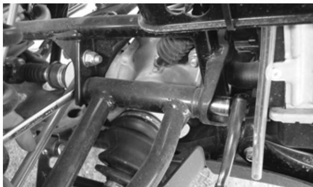
11. Remove the circlip from the ball joint; then remove the ball joint from the A-arm.
