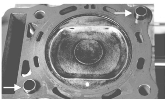
8. Install the four cylinder head cap screws and washers. Tighten only until snug.
