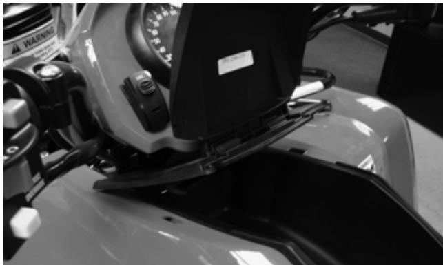
3. Remove the storage compartment box; then remove the seat.
