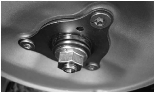
3. Identify the alignment marks on the shift arm and shift arm shaft to aid in installing; then remove the cap screw securing the shift arm to the shift arm shaft. Remove the shift arm from the shift arm shaft.
