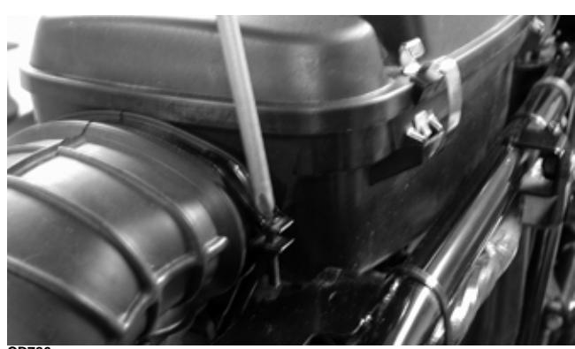
20. Connect the intake air temperature sensor connector.
