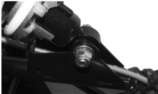
4. Using Spring Tool, compress the shock absorber spring, remove the retainer, and remove the spring.
